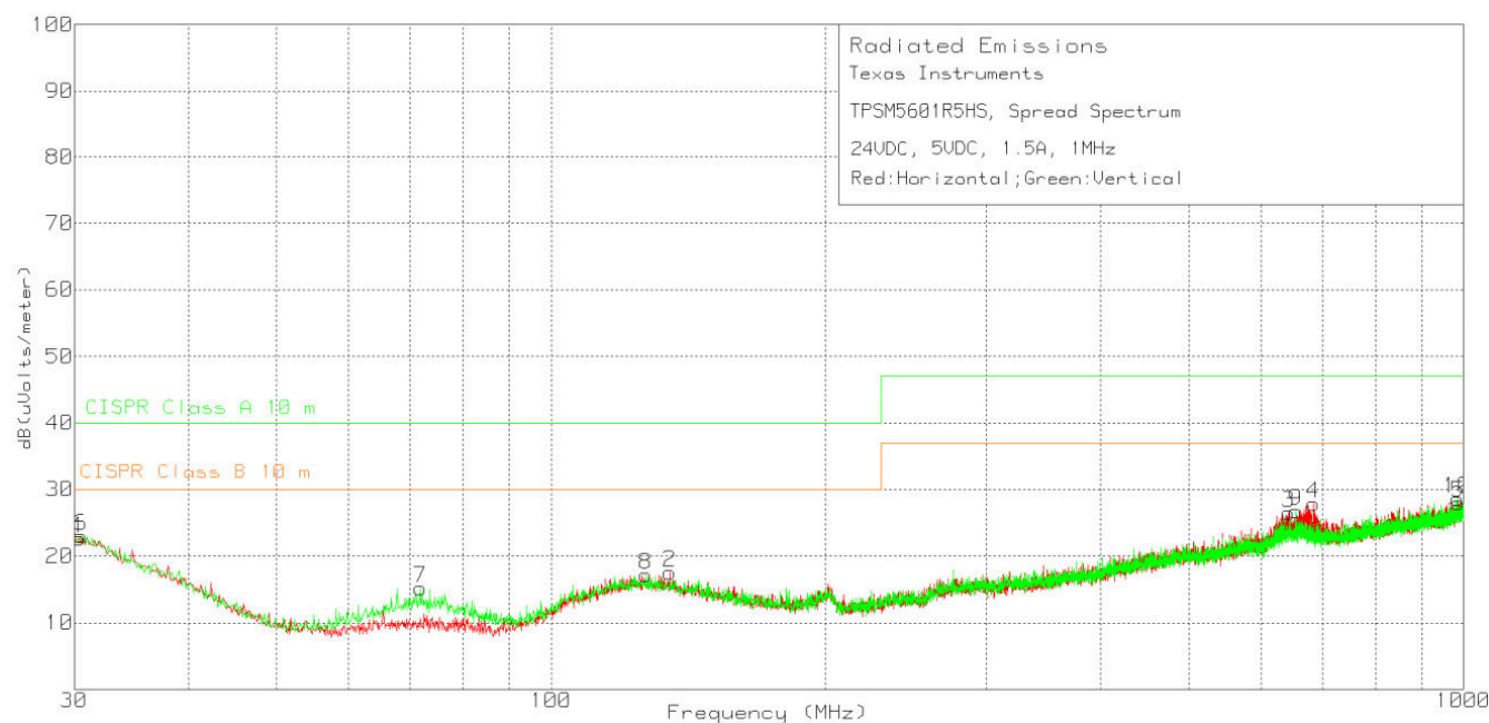
图 10-7. Radiated Emissions 24-V Input, 5-V Output, 1.5-A Load (Spread Spectrum)
