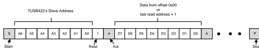
图 7. I2C Read Without Repeated Start
