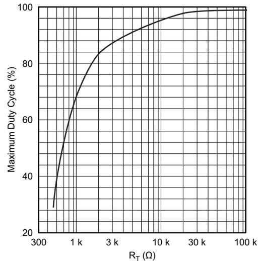
图 7-5. Maximum Duty Cycle vs Timing Resistance
