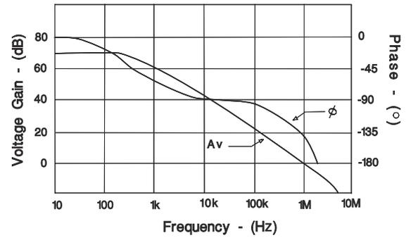
**图 6-2. Error Amplifier Open-Loop Frequency Response**
