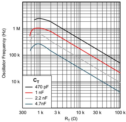
图 7-4. Oscillator Frequency vs Timing Resistance
