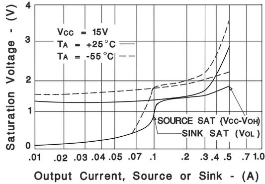
**图 6-1. Output Saturation Characteristics**
