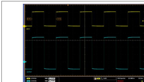
图 9-14. PWM Input (Yellow) and Driver Output (Blue)
