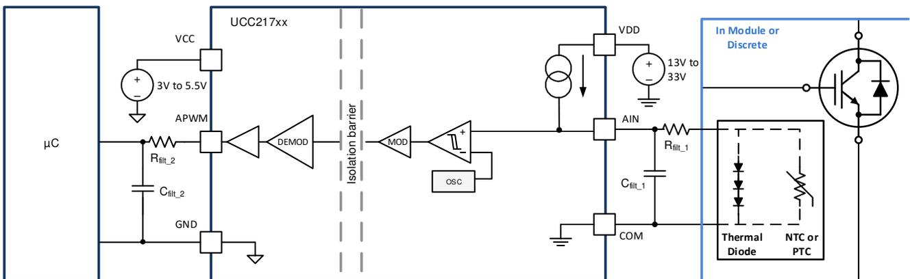
图 9-8. APWM Channel with Filtered Output
