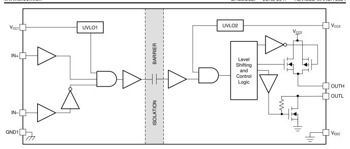
图 8-3. Functional Block Diagram — Split Output (UCC53x0S)
