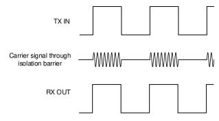
图 8-2. On-Off Keying (OOK) Based Modulation Scheme
