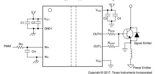
图 9-1. Typical Application Circuit for UCC53x0S to Drive IGBT
