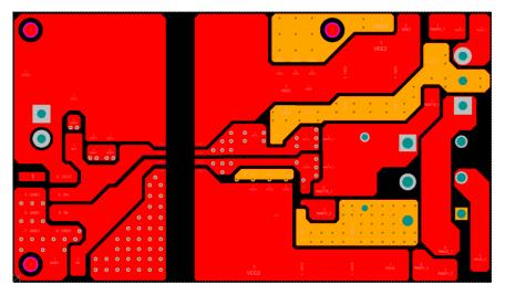
图 11-2. Top-Layer Traces and Copper
