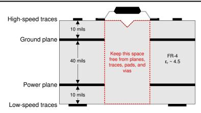
图 11-5. Recommended Layer Stack
