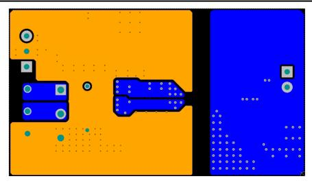
图 11-3. Bottom-Layer Traces and Copper (Flipped)
