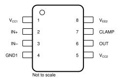
图 5-2. UCC5310M and UCC5350M 8-Pin SOIC Top View
