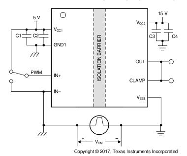
图 7-4. CMTI Test Circuit for Miller Clamp (UCC53x0M)
