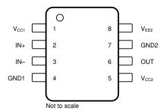
图 5-3. UCC5320E and UCC5390E 8-Pin SOIC Top View
