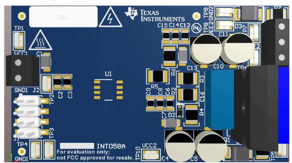
The location of the PCB cutout between primary side and secondary sides ensures isolation performance.
