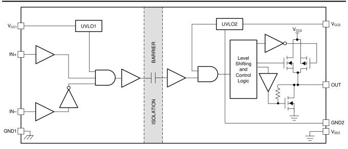
图 8-5. Functional Block Diagram — UVLO With Respect to GND2 (UCC53x0E)
