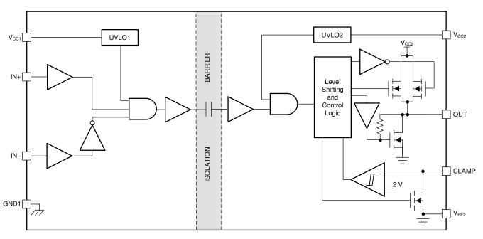
图 8-4. Functional Block Diagram — Miller Clamp (UCC53x0M)
