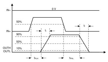
图 7-1. OUTH and OUTL Propagation Delay, Noninverting Configuration
