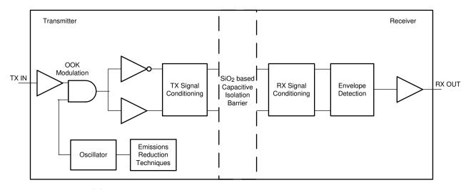
图 8-1. Conceptual Block Diagram of a Capacitive Data Channel
