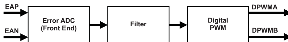
图 6-1. Simple Digital Power Configuration
