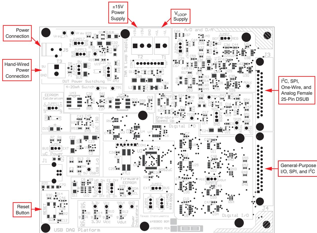
Figure 26. Connector Definition
