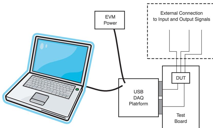
**Figure 2. Hardware Setup for the USB DAQ Platform**
