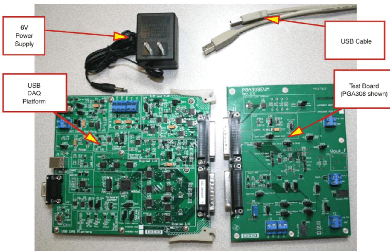
Figure 1. Typical Hardware Included with the USB DAQ Platform
