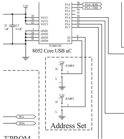
Figure 8. Digital I/O Area—Address Select
