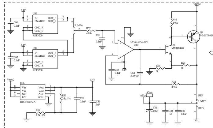
Figure 20. DAC, ADC, and INA—Reference
