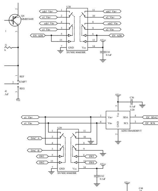
Figure 21. DAC, ADC, and INA—ADS1100 a1 Connections
