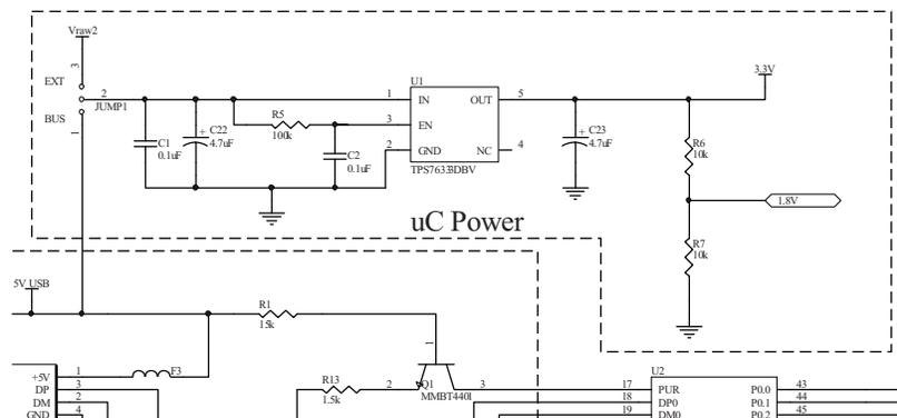
Figure 9. Microcontroller Power
