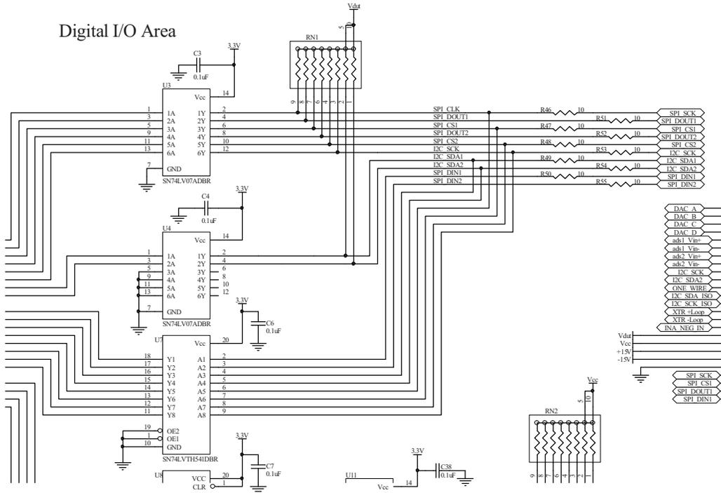
Figure 5. Digital I/O Area—I<sup>2</sup>C and SPI
