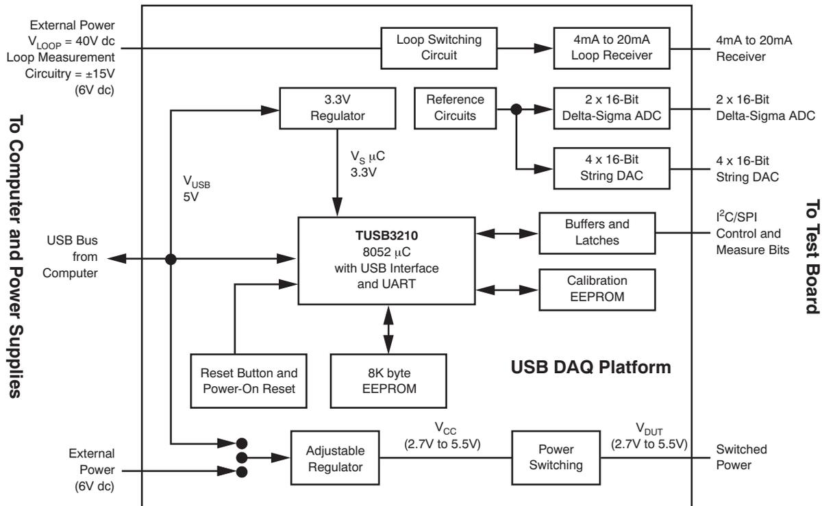
Figure 3. USB DAQ Platform Block Diagram
