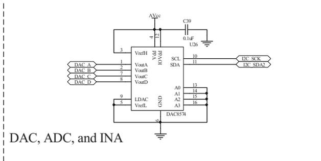
Figure 23. DAC, ADC, and INA—DAC8574
