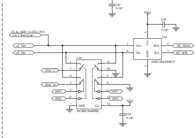
Figure 22. DAC, ADC, and INA—ADS1100 a2 Connections
