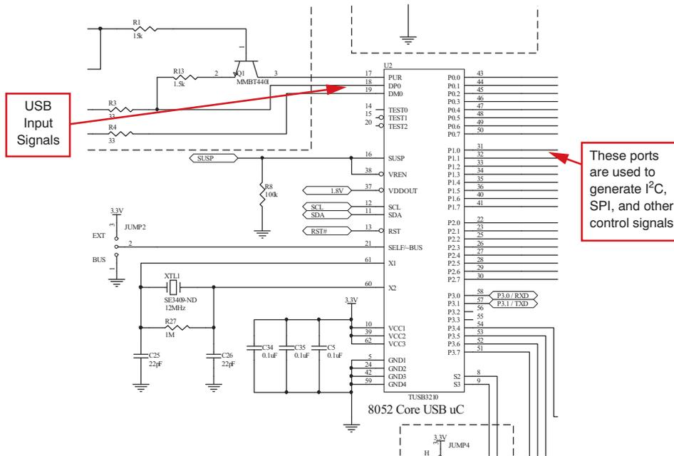
Figure 4. Digital I/O Area—Microcontroller
