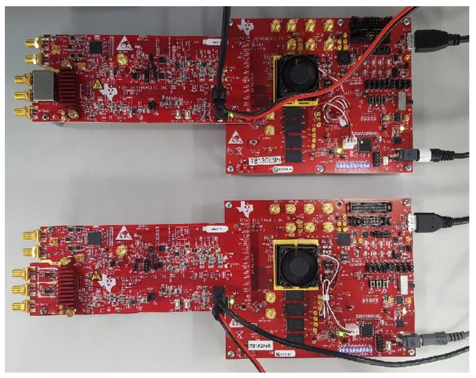
Figure 2. TSW40RF82 and TSW14J56 Setup
