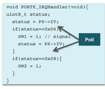
**PxIV** it will get the number  $(2^*(n+1))$  where *n* is the pin number of the lowest bit with a pending interrupt
