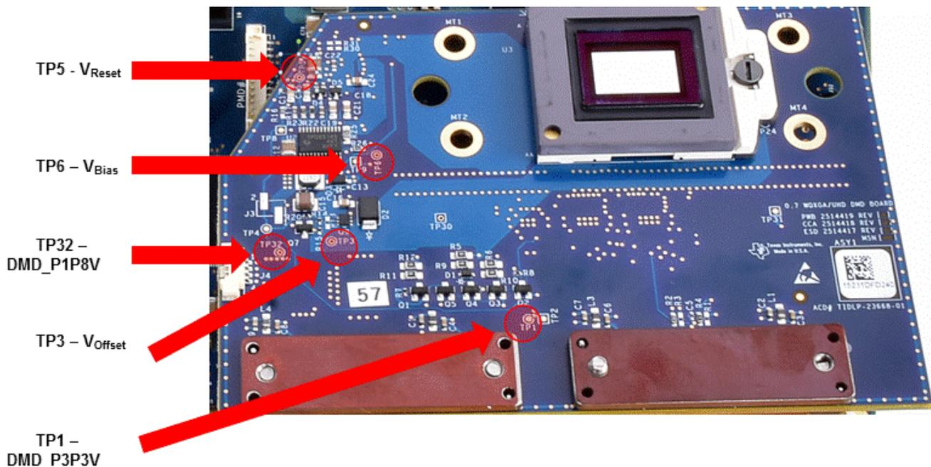
Figure 12. DMD Board Test Points
