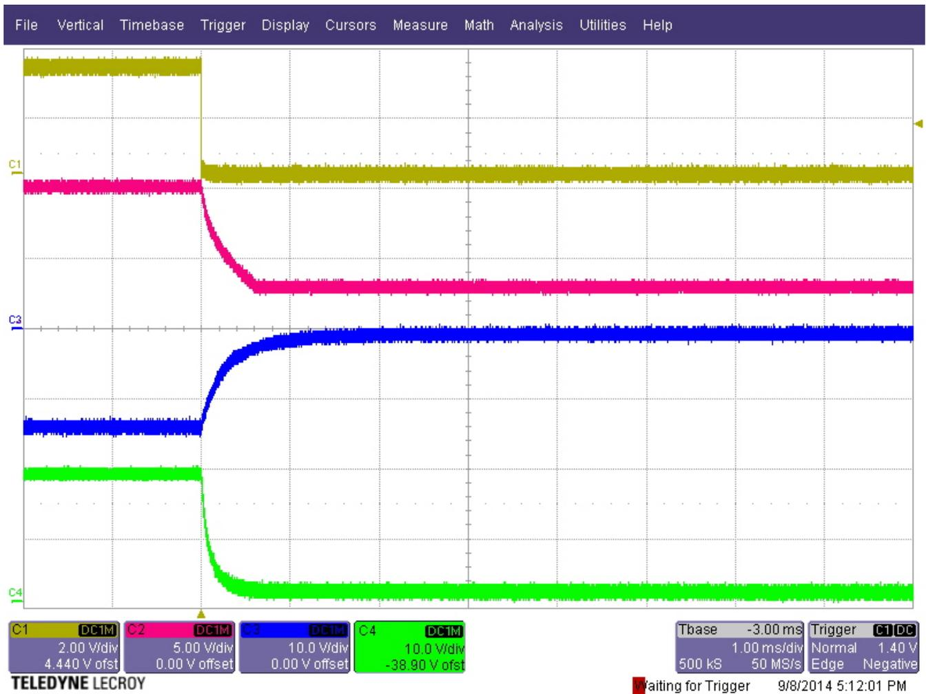
Figure 15. DMD Shut-down Power Sequencing
