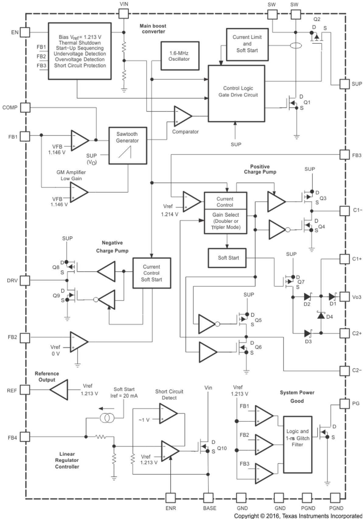
Figure 5. TPS65145 Block Diagram
