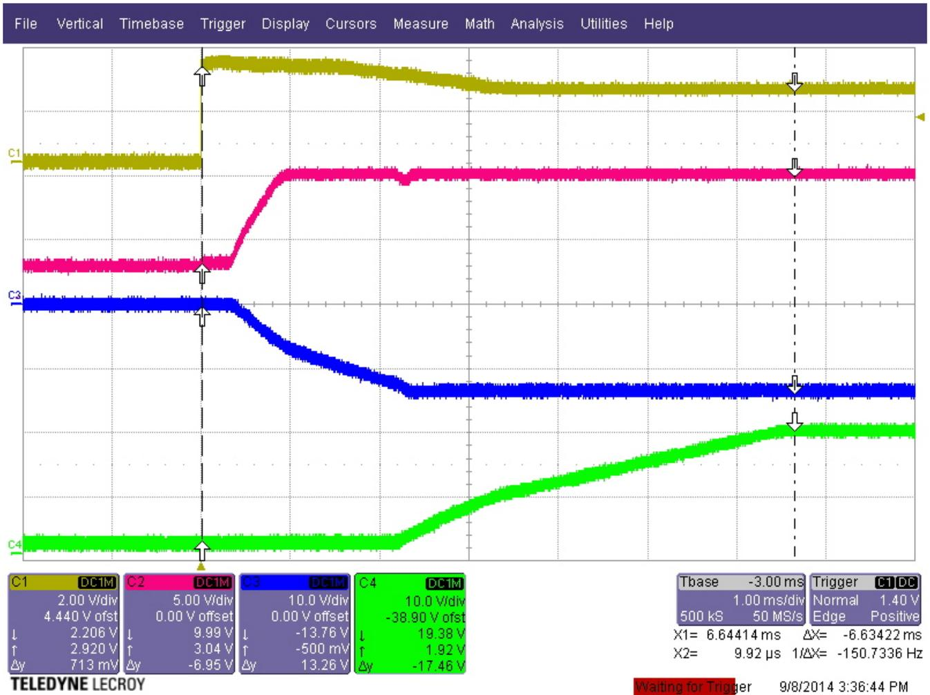
Figure 14. DMD Start-up Power Sequencing
