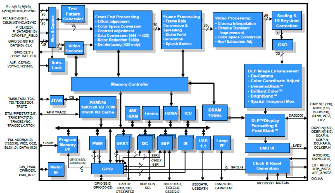
Figure 3. DLPC4422 Block Diagram
