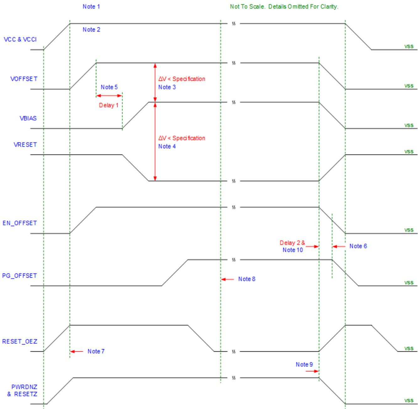
Figure 13. DMD Power Supply Timing Diagram
