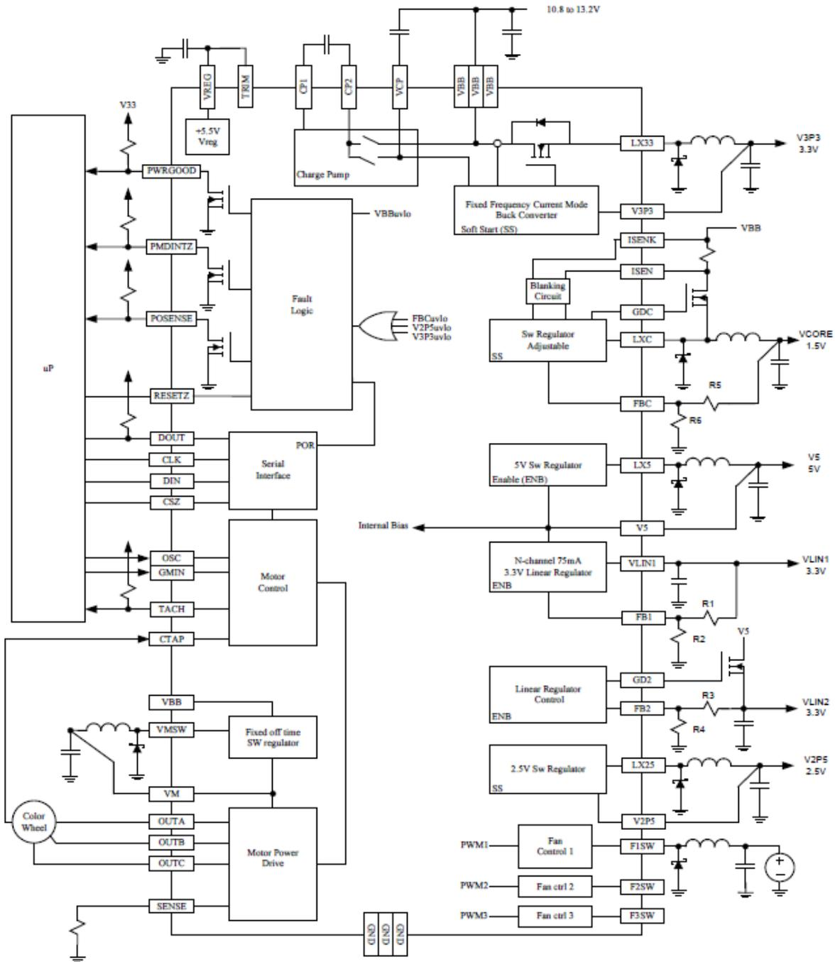
Figure 4. DLPA100 Block Diagram
