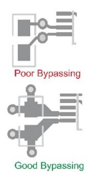
Figure 3. Decoupling Capacitor Example
