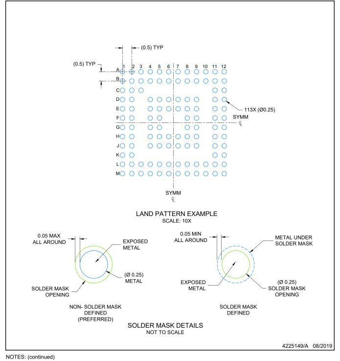
3. Final dimensions may vary due to manufacturing tolerance considerations and also routing constraints. Refer to Texas Instruments Literature number SNVA009 (www.ti.com/lit/snva009).
