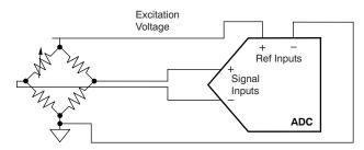
Figure 2. Ratiometric Measurement of Load Cell with an ADC
