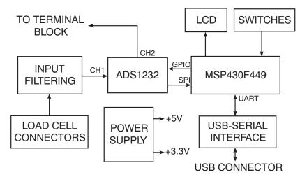
Figure 5. Block Diagram of the ADS1232REF Weigh Scale Reference Design
