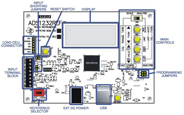
Figure 6. ADS1232REF Weigh Scale Reference Design Layout
