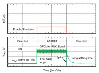
Figure 2. Output Results for Improperly Configured Circuit
