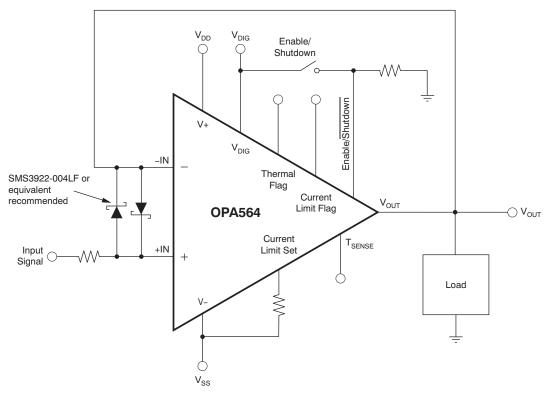
Figure 8. Dual Supply, DC-Connected Load Unity-Gain Follower
