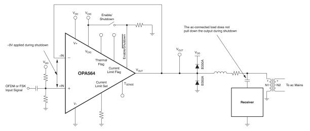
Figure 3. Unity-Gain Powerline Communications Line Driver with AC-Coupled Load
