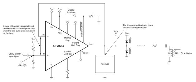
Figure 1. Unity-Gain Powerline Communications Line Driver with DC-Coupled Load
