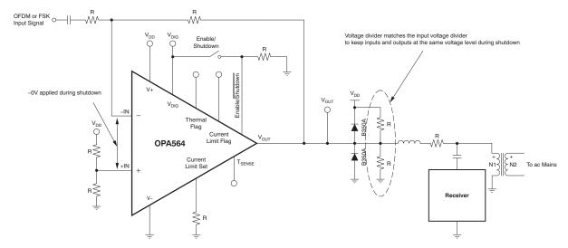
Figure 6. AC-Coupled, Inverting Gain Powerline Communications Line Driver with AC-Coupled Load and Voltage Divider
