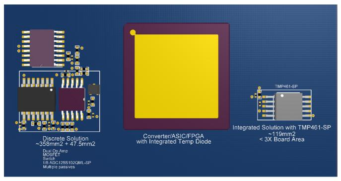
Figure 3. Discrete Solution vs. TMP461-SP Layout
