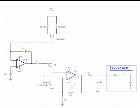
Figure 1. Discrete Temperature Sensing Circuit
