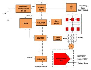
Figure 1. Typical HV Traction Inverter
