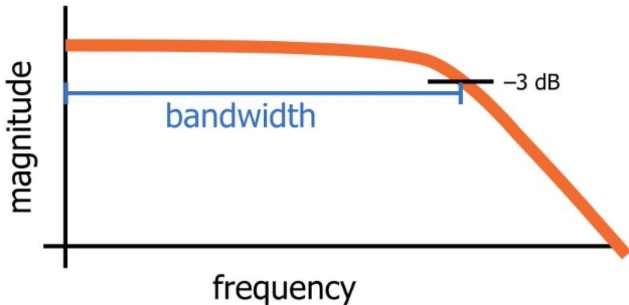
Figure 1. Bandwidth of Low-Pass Filter
