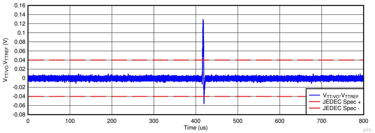
**Figure 7-6. The Difference Between VTT/VO and VTTREF, Exceeding  $\pm 40\text{mV}$**
