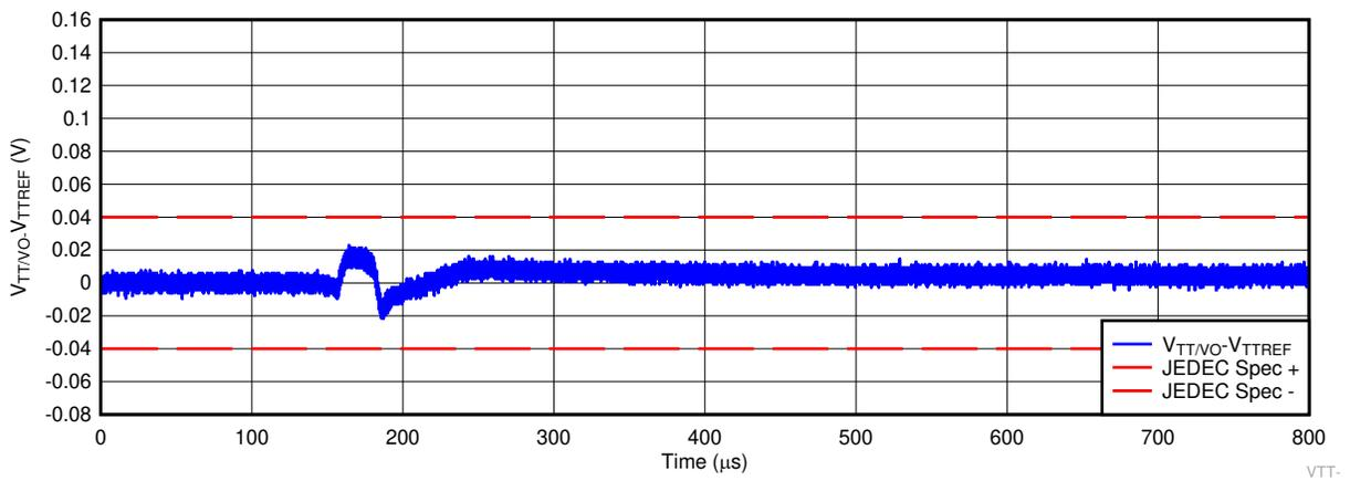
Figure 7-3. The Difference Between  $V_{TT}/V_0$  and  $V_{TTREF}$  is Approximately  $\pm 20\text{mV}$
