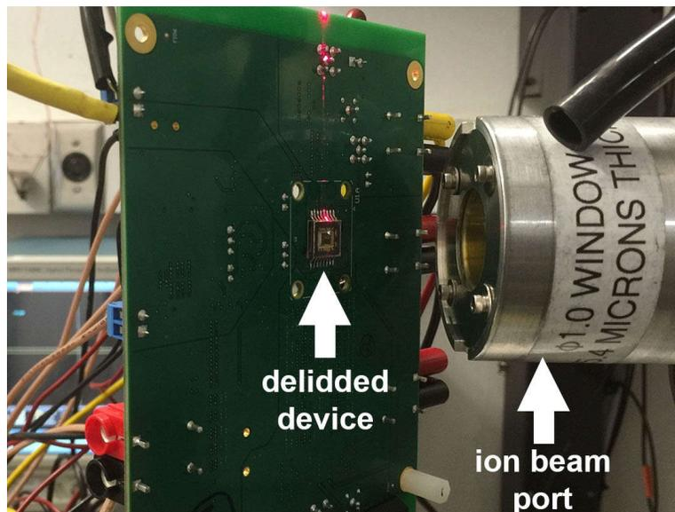
Figure 4-1. Photograph of the TPS7H3301-SP Evaluation Board Mounted in Front of the Heavy Ion Beam Exit Port at the TAMU Accelerator Facility
