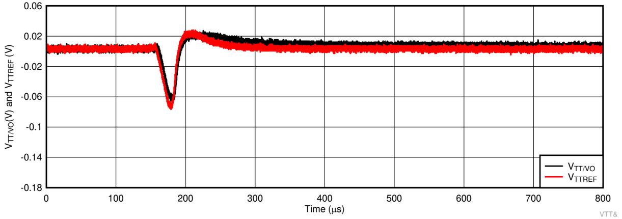
Figure 7-2.  $V_{TT}/V_0$  and  $V_{TTREF}$  Signals Track During the Event
