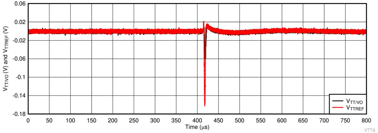
**Figure 7-5. VTT/VO and VTTREF Signals Tracking With Some Disparities During the Event**
