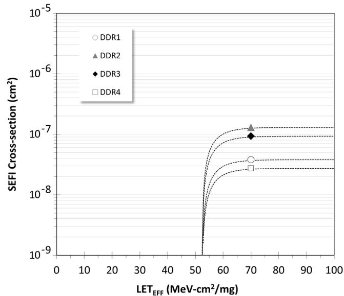
**Figure 8-1. SEFI Cross Sections for TPS7H3301-SP as a Function of  $LET_{EFF}$**
