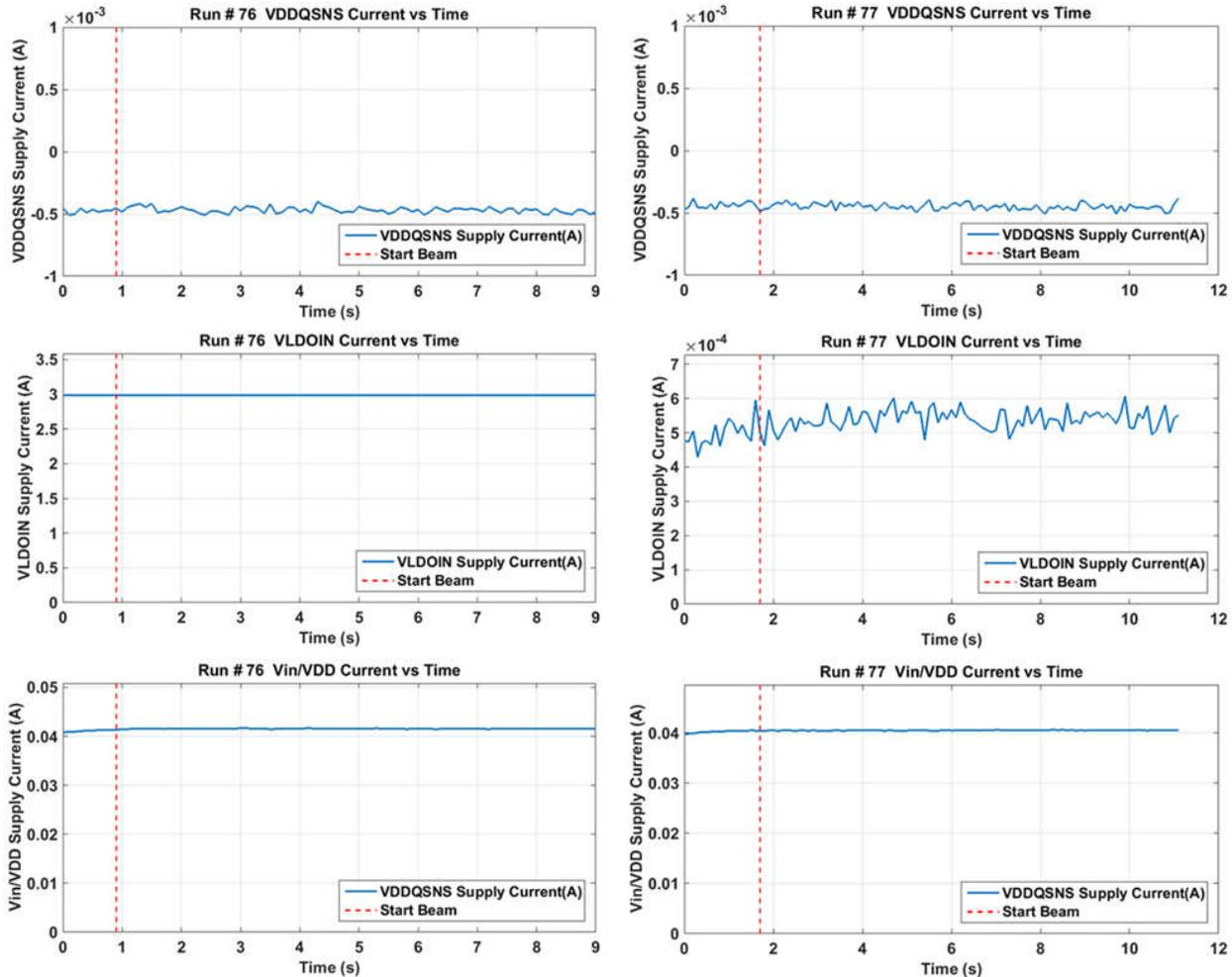
Figure 7-1. SEL Current versus Time (I Versus t) Data in DDR1 Mode for Sourcing (Left) and Sinking 3A (Right)
