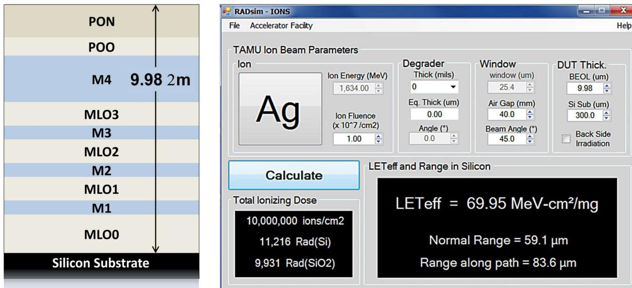
Figure 5-1. Layer Stack of TPS7H3301-SP (Left) and RADsim-IONS Program (Right) Used to Determine Key Ion Parameters
