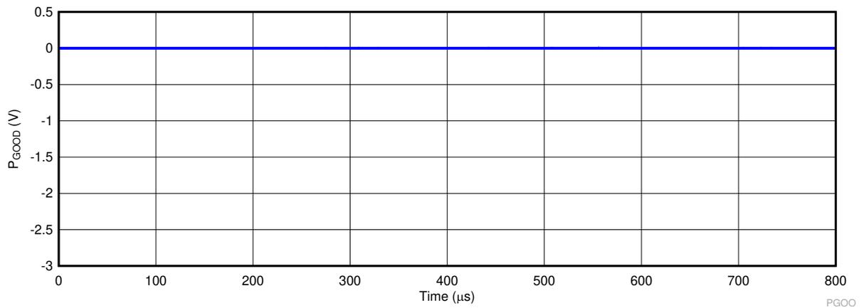
Figure 7-4.  $P_{GOOD}$  Signal is Not Triggered Since the Set Was Not Big Enough to Cause a Tracking Error
