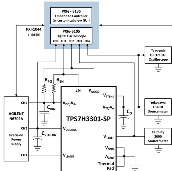
**Figure 6-1. Block Diagram of Heavy-Ion SEE Test Set-Up With the TPS7H3301-SP on a TPS7H3301EVM-CVAL (HREL022) Evaluation Board**
