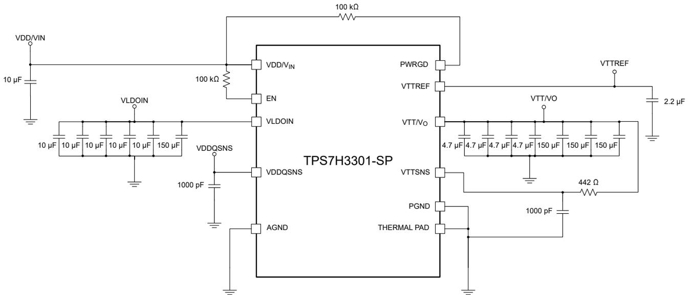
**Figure 3-3. Schematic of the Prototype TPS7H3301EVM-CVAL (HREL022) Evaluation Board Used to Perform the SEE Tests on the TPS7H3301-SP Devices**
