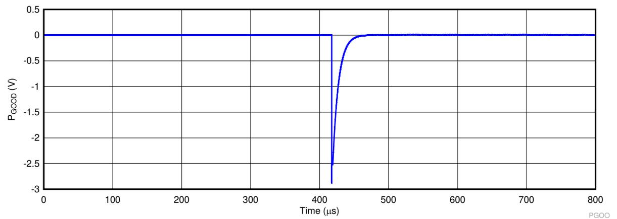
**Figure 7-7. The Corresponding P<sub>GOOD</sub> Signal Which Flags the Tracking Error Between VTT/VO and VTTREF**
