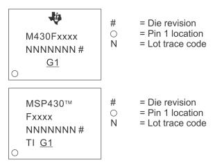
NOTE: Package marking with "TM" applies only to devices released after 2011.
