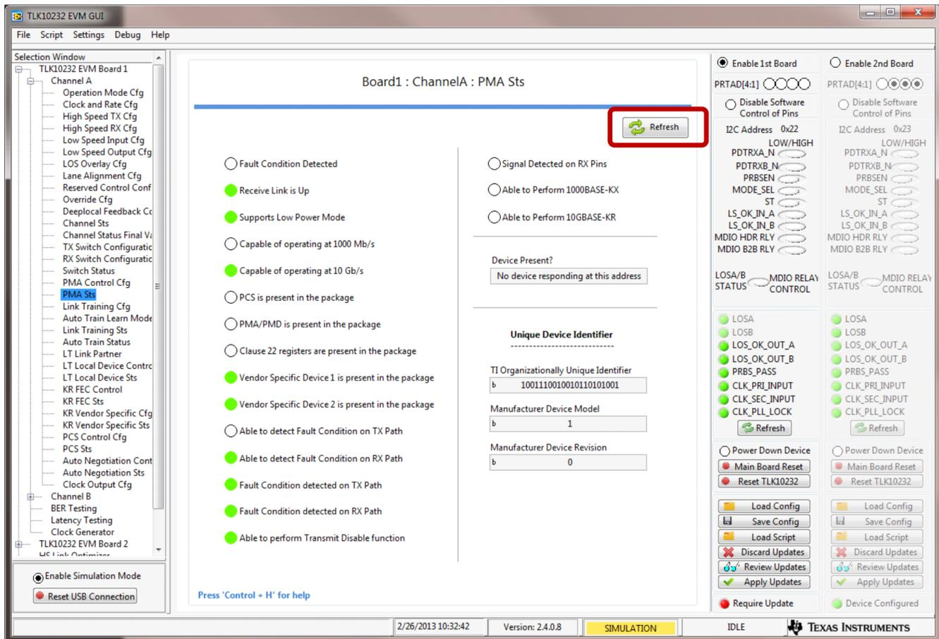
Figure 7. TLK10232 EVM GUI High-Level Device Status Windows
