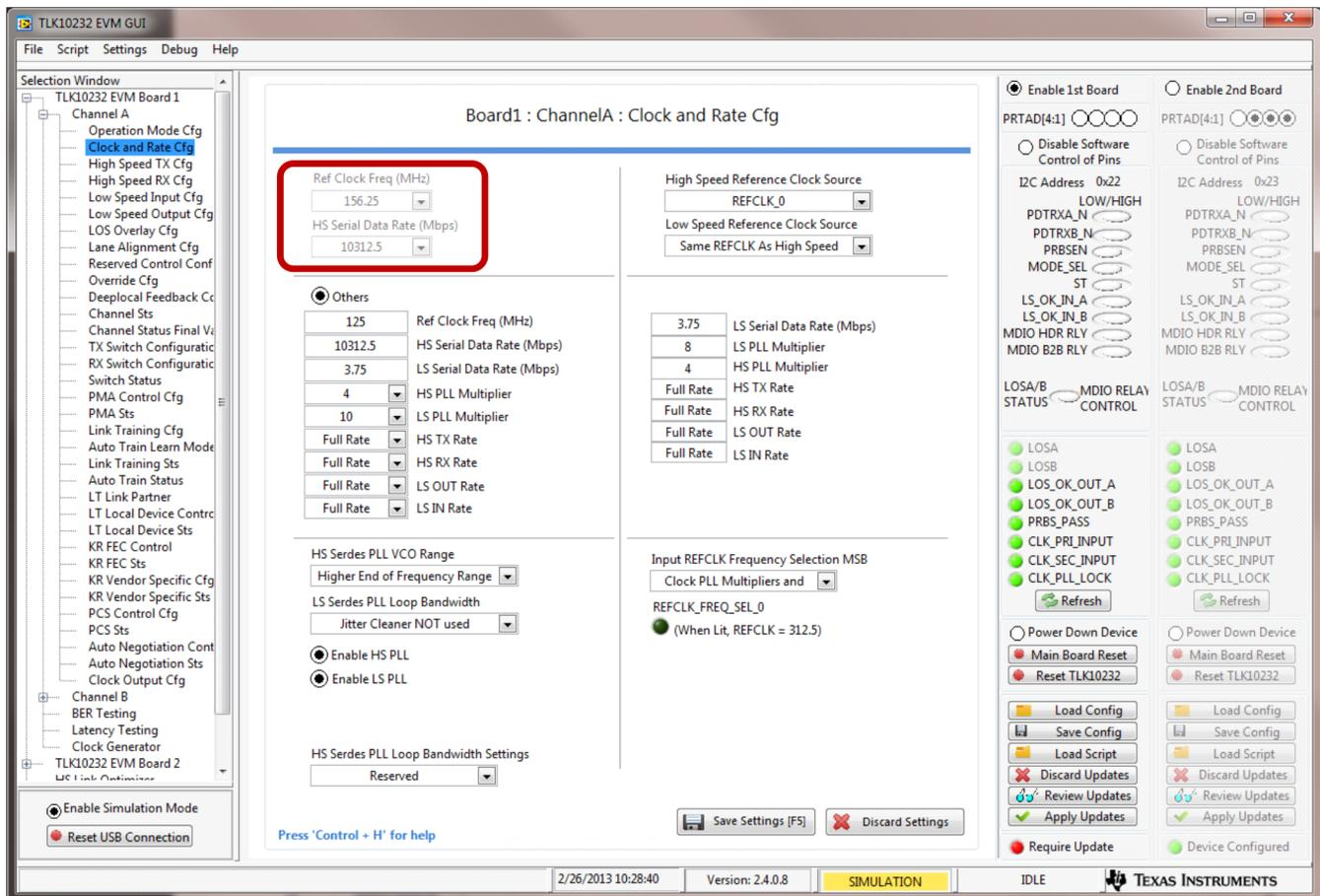
Figure 6. TLK10232 EVM GUI High-Level Device Configuration
