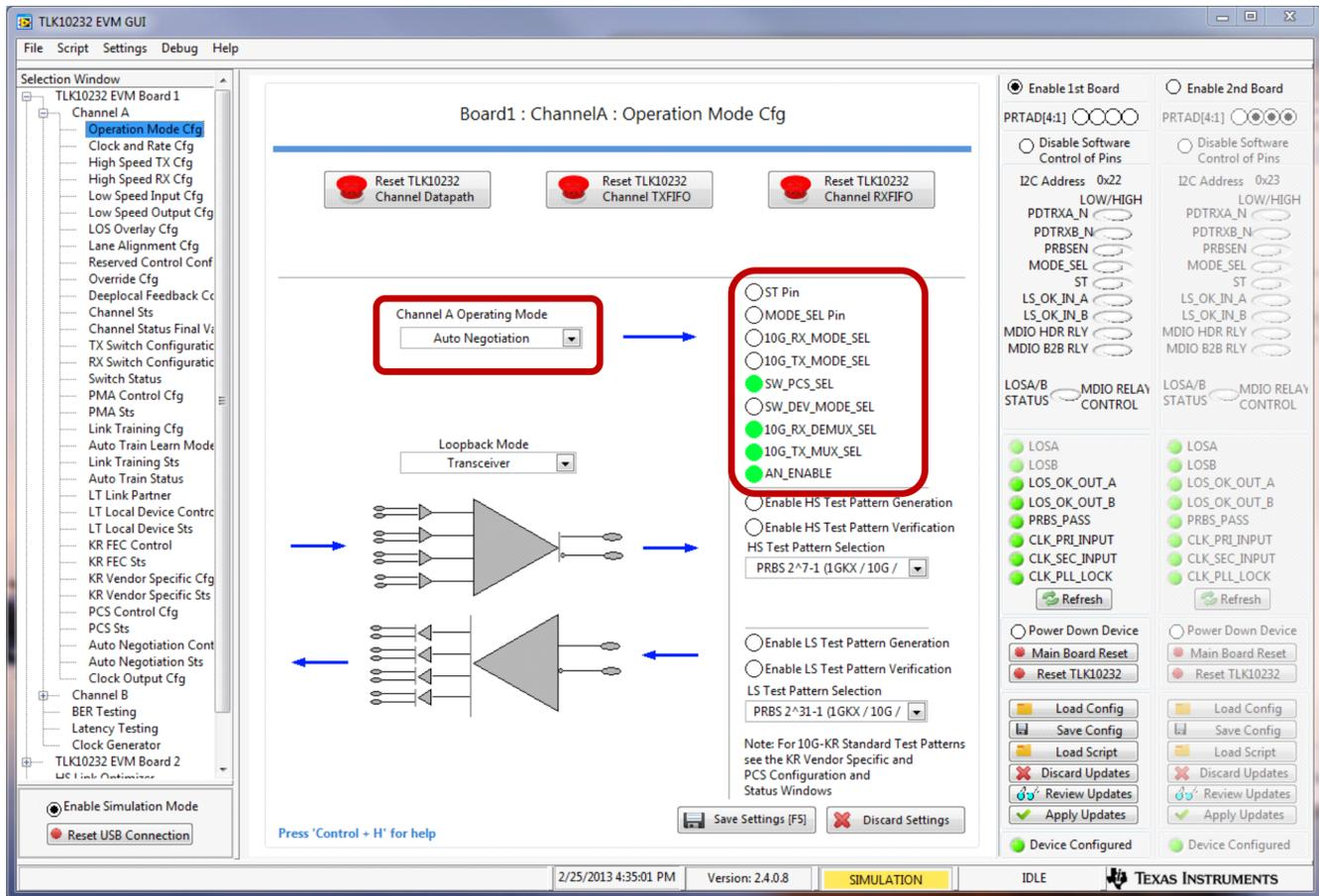
Figure 4. TLK10232 EVM GUI Operating Mode Configuration
