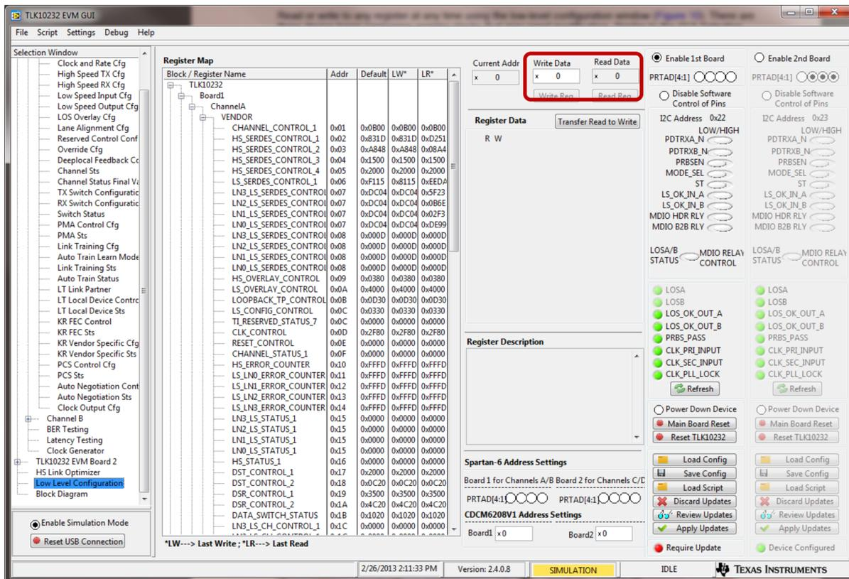
Figure 10. TLK10232 EVM GUI Low-Level Device Configuration
