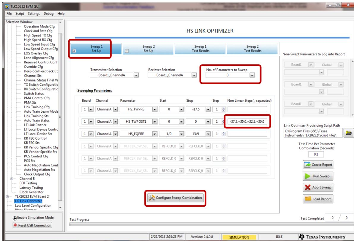
Figure 13. TLK10232 EVM GUI High-Speed Link Optimizer Setup
