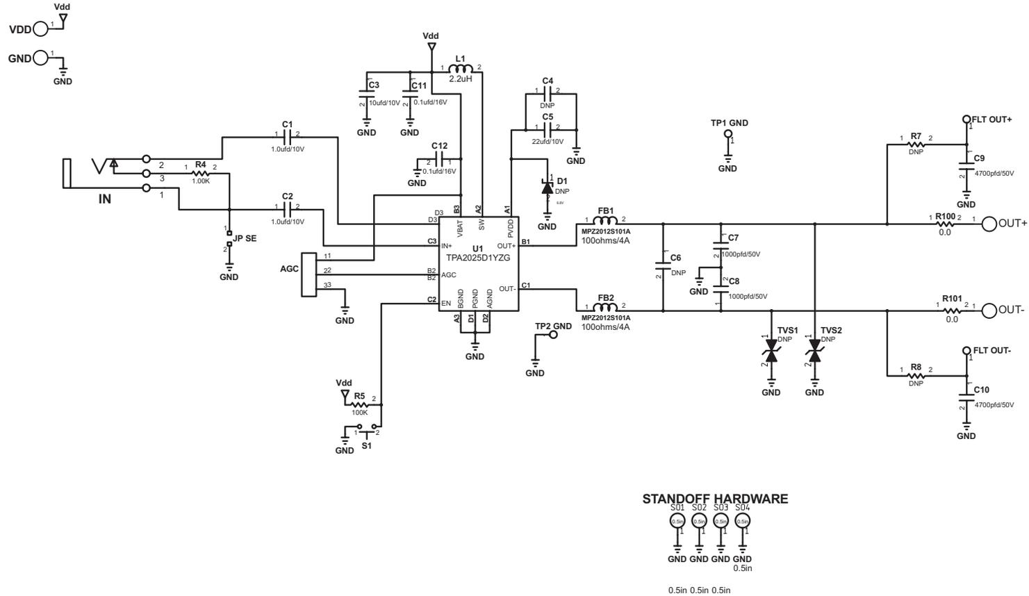
Figure 1. TPA2025D1EVM Schematic
