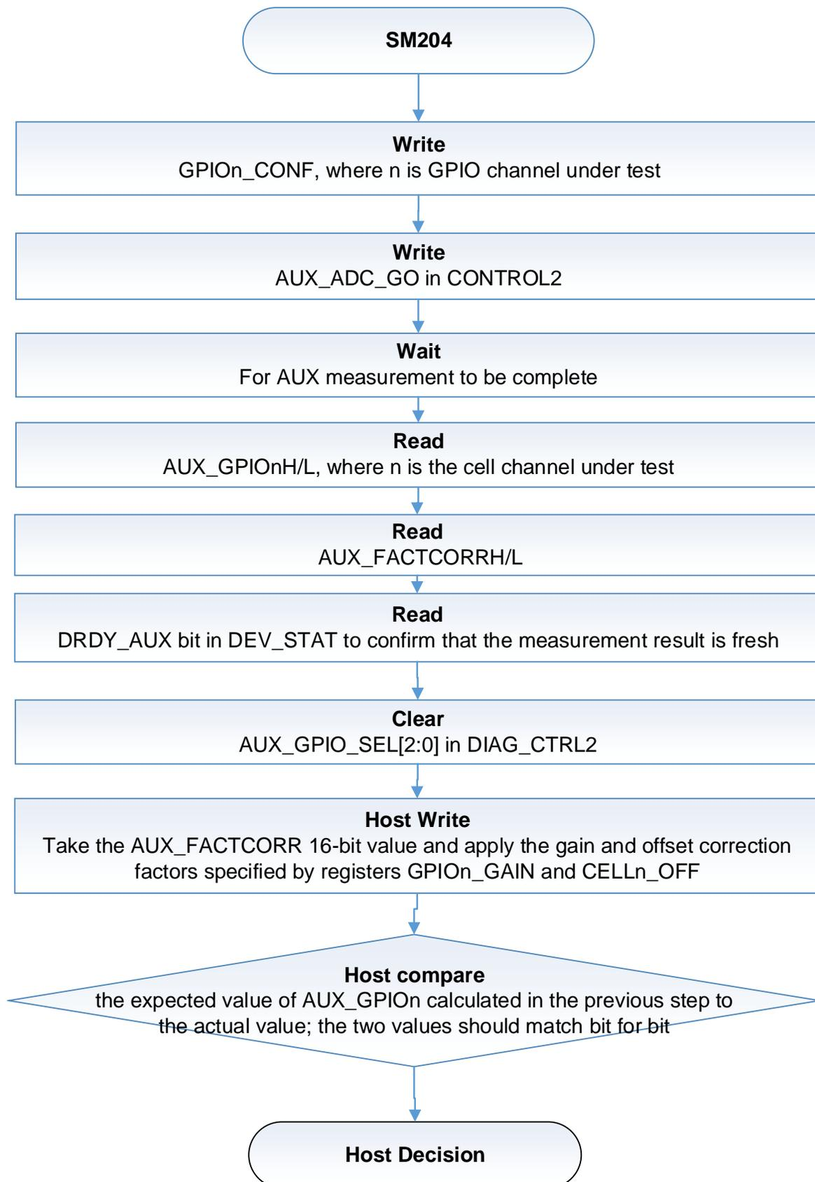
**Figure 14. SM204: AUXADC Gain Offset and Output Register Check**
