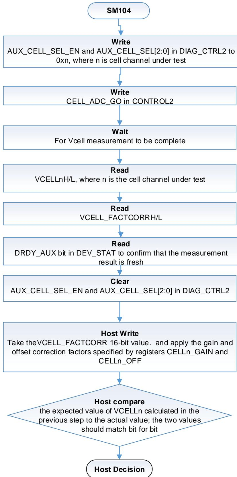
Figure 7. SM104: VCell Gain and Offset Register Check
