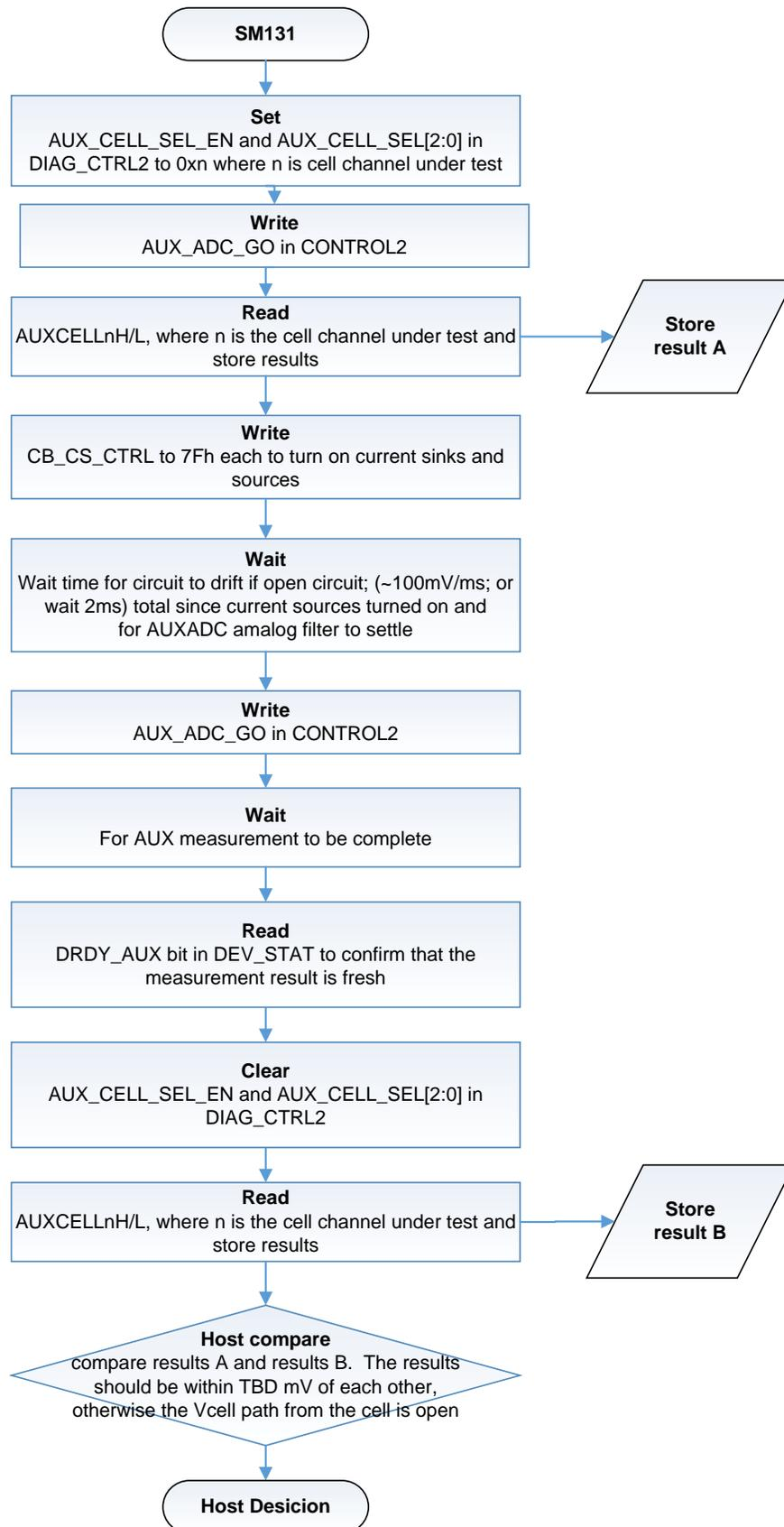
Figure 9. SM131: CB Path and Pin Open Check
