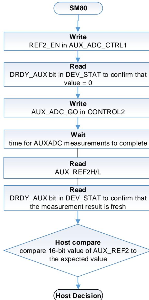
**Figure 5. SM80: REF1 vs REF2 Accuracy measurement**
