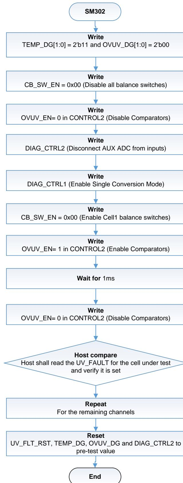
**Figure 18. SM302: OV/UV Multiplexor Selector integrity**
