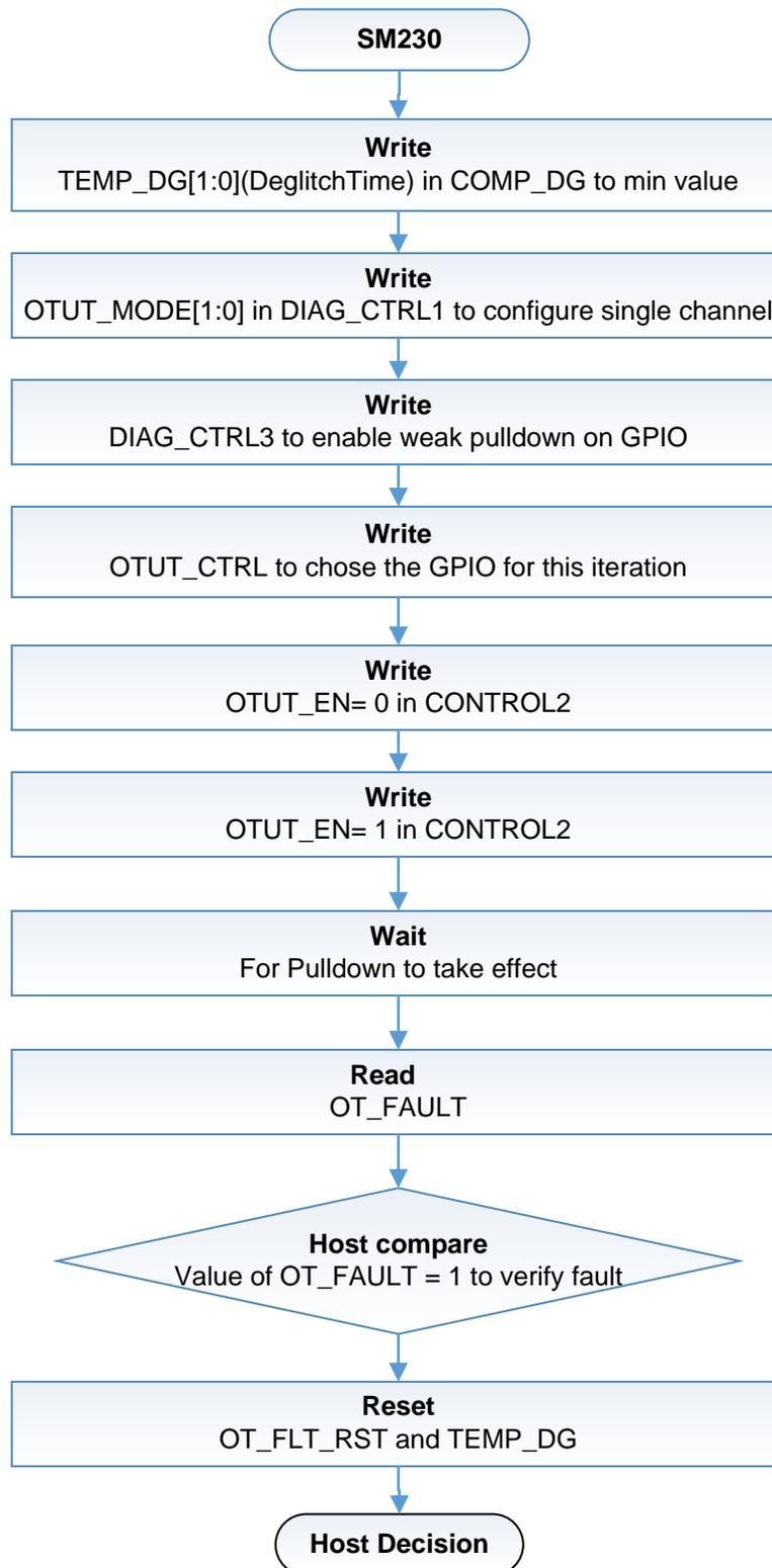
**Figure 15. SM230: GPIO Pin Open Check**
