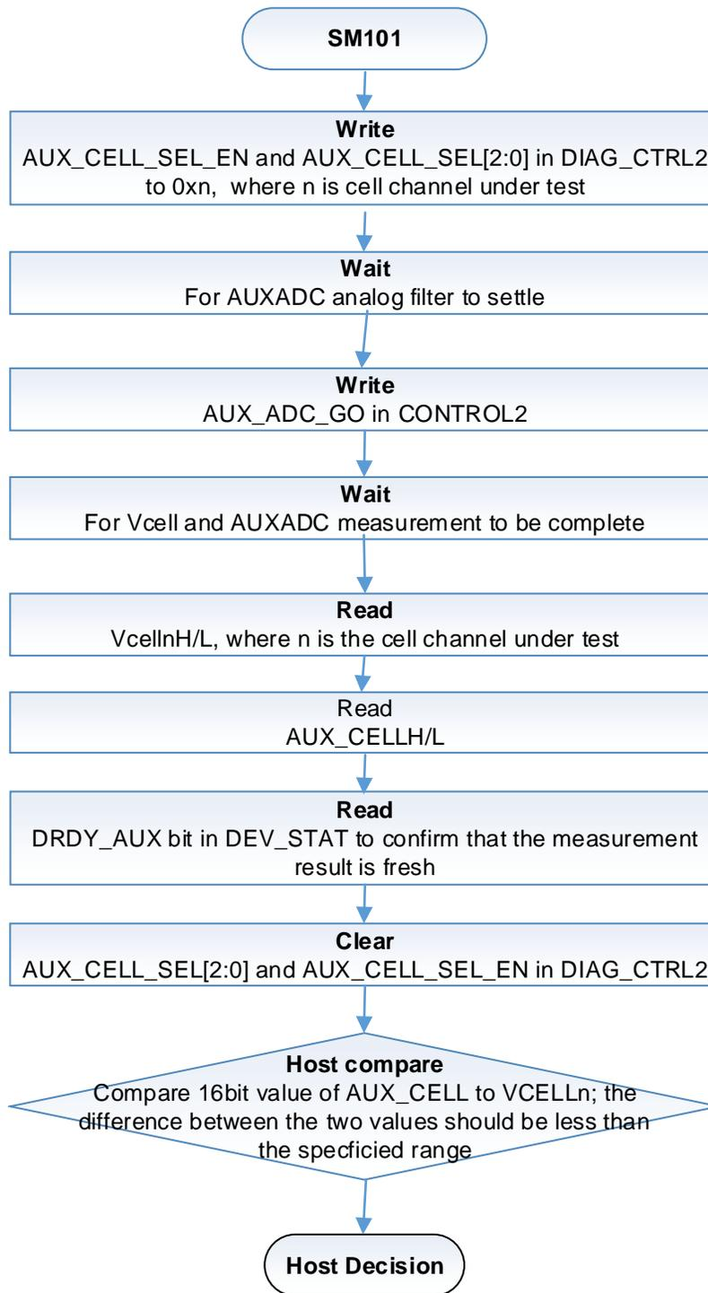
Figure 6. SM101: VCell ADC Path Accuracy Check
