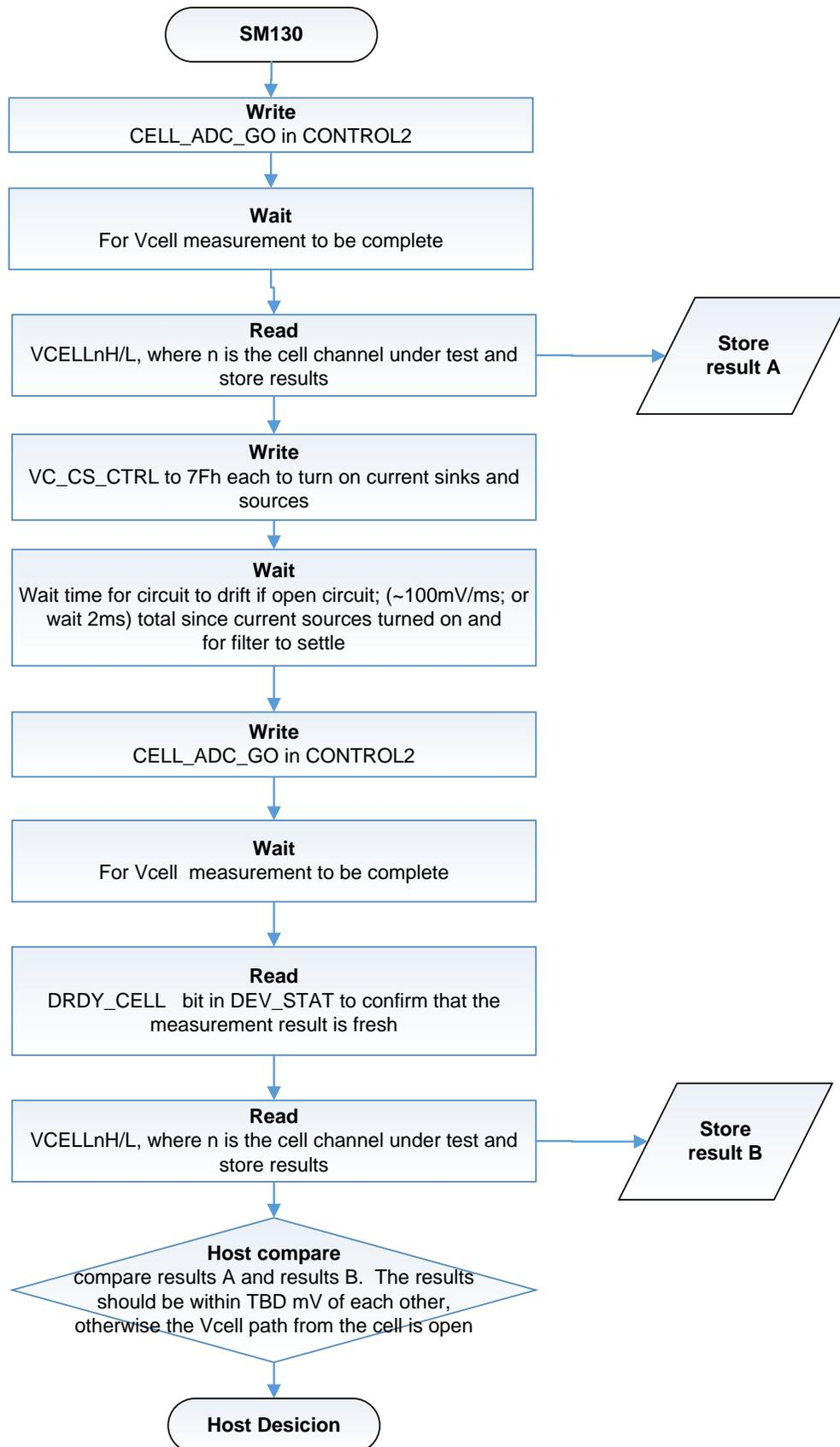
Figure 8. SM130: VC Path and Pin Open Check
