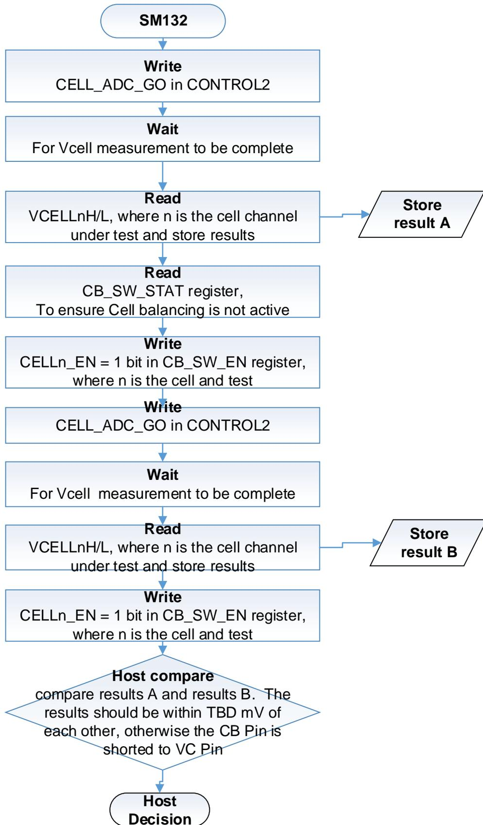
Figure 10. SM132: VC and CB Pin Short Check
