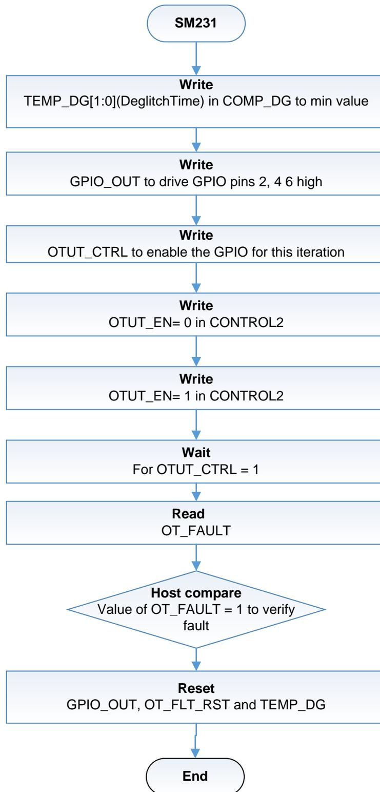
Figure 16. SM231: GPIO Multiplexer and Pin Short Check
