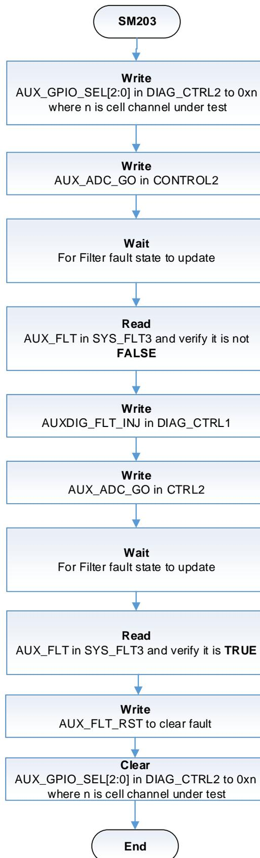
**Figure 13. SM203: AUXADC Redundant Digital Filter Fault Injection**
