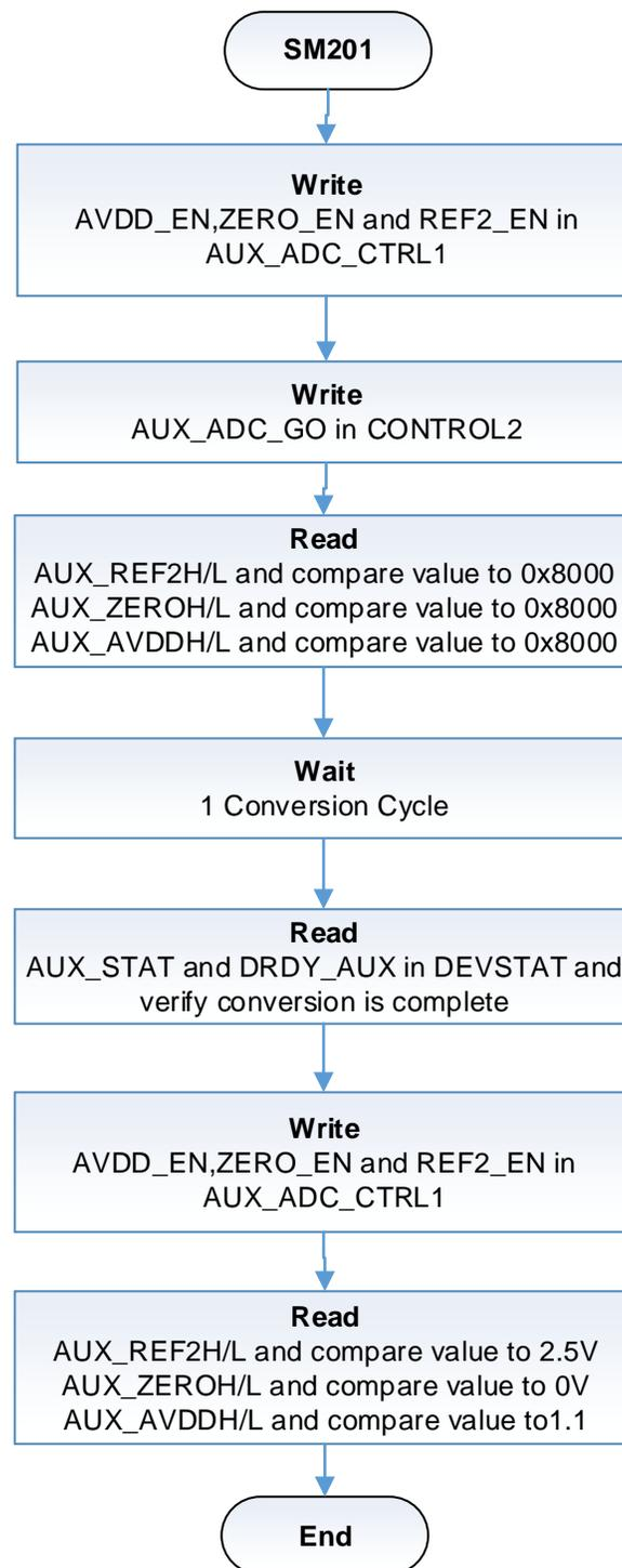
**Figure 11. SM201: AUXADC Linearity Check**
