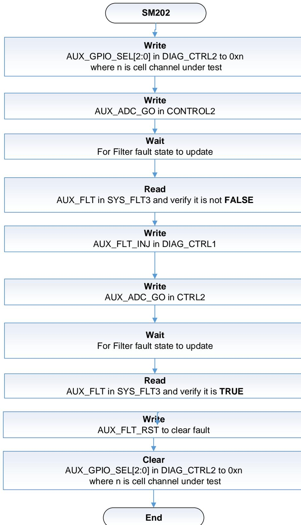
**Figure 12. SM202: AUXADC Digital Circuit Check**
