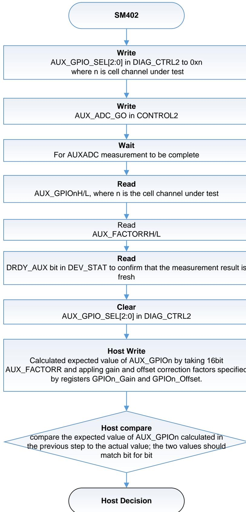
Figure 19. SM402: OT/UT Multiplexor Selector Integrity
