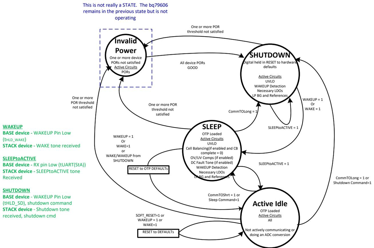
The BQ79606A-Q1 always operates in one of four modes. The mode depends on the VBAT voltage and the operational requirements of the system. A high level description of the modes is as follows:
