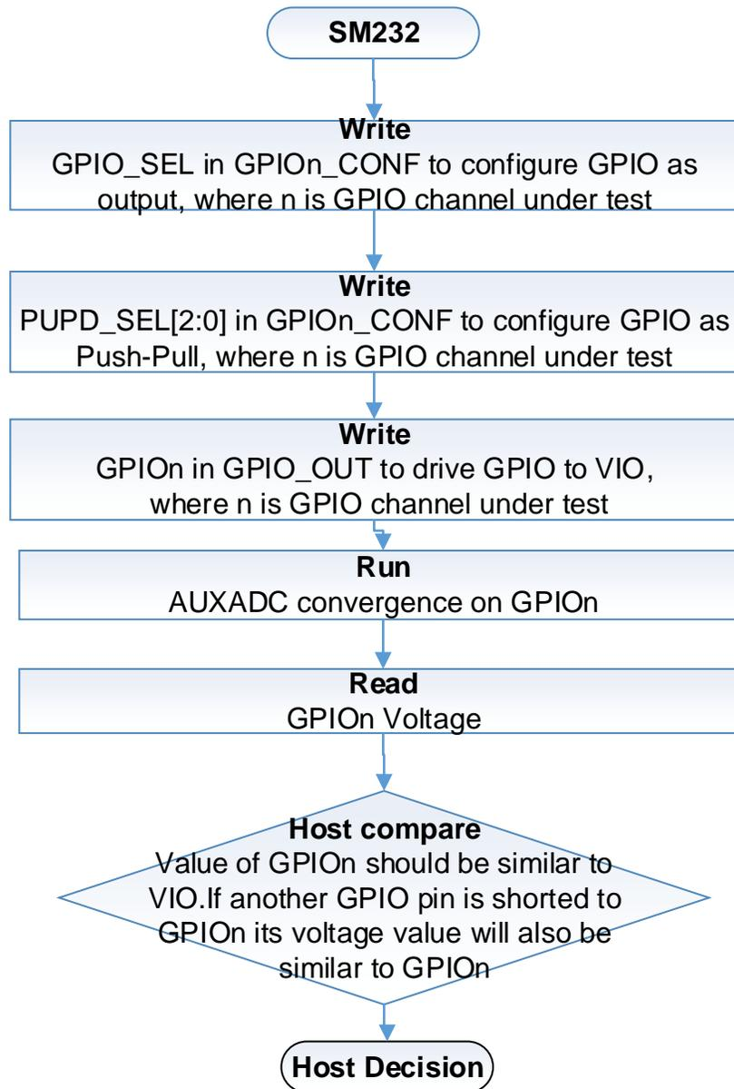
**Figure 17. SM232: AUXMUX GPIO Check**
