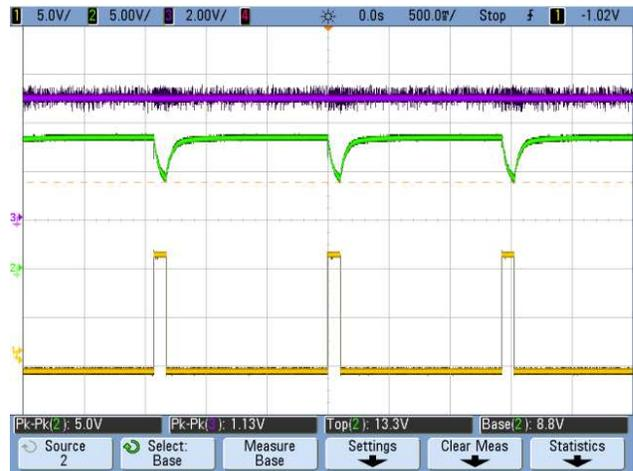
Figure 18. 480 VAC: No Load on 5-V Output, 12-V Load Transient
