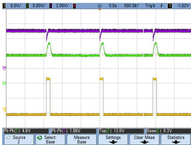
**Figure 15. 90 VAC: Full Load on 12-V Output, 5-V Load Transient**
