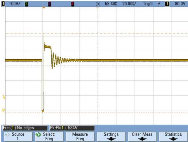
Figure 28. 240-VAC Input: 230 No Load (Zoom)
