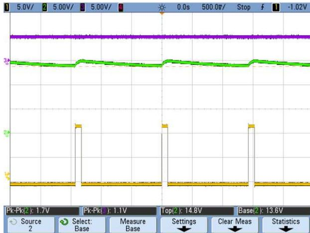
**Figure 13. 90 VAC: No Load on 12-V Output, 5-V Load Transient**
