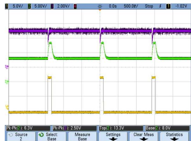
**Figure 16. 480 VAC: Full Load on 12-V Output, 5-V Load Transient**
