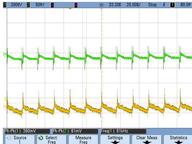
Figure 37. 480-V Full Load Output Ripple
