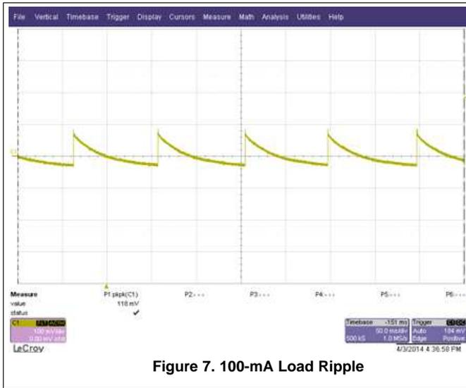
Figure 7. 100-mA Load Ripple
