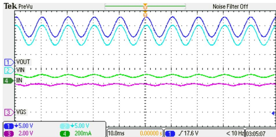
**Figure 4. Stable VGS With 1- $\mu$ F Input Capacitor and 0.1- $\mu$ F Output Capacitor**
