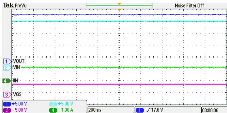
Figure 2. LM5050-1 Operation Showing  $V_{IN}$  (20 VDC),  $V_{OUT}$ ,  $V_{GS}$ , and  $I_{IN}$  (1.2 A)
