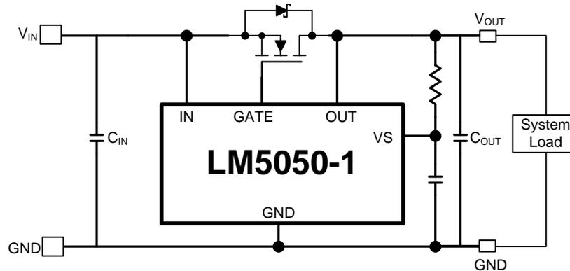
Figure 1. LM5050-1 Application Circuit
