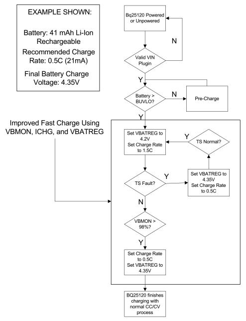
Figure 1. Improved Fast Charge Flow Chart Using the bq25120 Features
