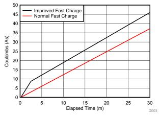
Figure 4. Comparison of Standard vs Improved Fast Charging
