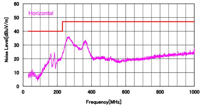
**Figure 8. Radiated Noise With Bead and RC Snubber**
