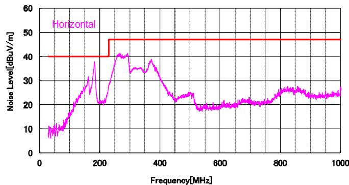
Figure 6. Radiated Noise With the RC Snubber
