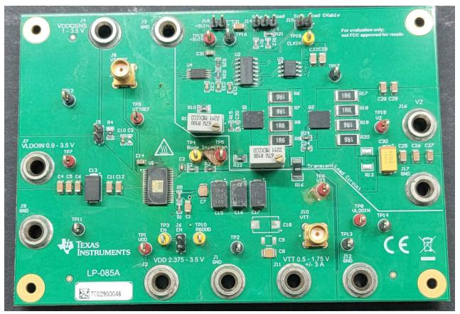
Figure 3-2. TPS7H3302-SEP Evaluation Board Top View
