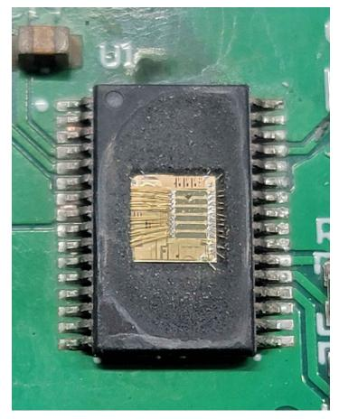
Figure 3-1. Photograph of the TPS7H3302-SEP Space DDR Termination Regulator Delidded
