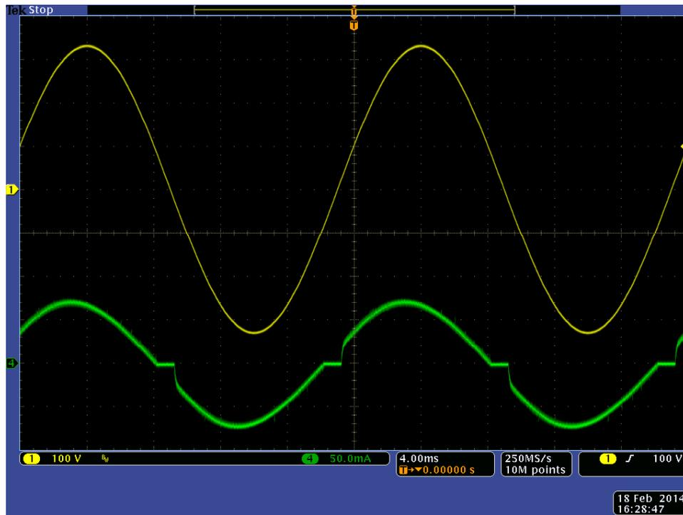
Figure 6. Input Voltage (Top) and Input Current (Bottom)
