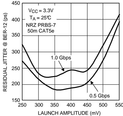
Figure 2. DS15EA101 Output Residual Jitter as a Function of Launch Amplitude
