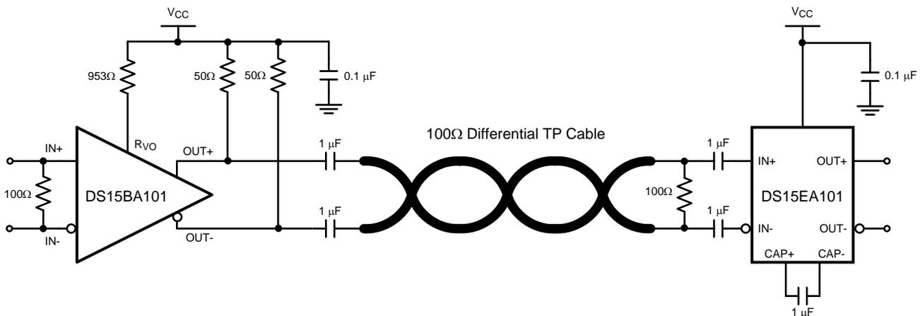
Figure 7. Cable Extender Chipset Connection Diagram for 100 $\Omega$  Differential Balanced Cables
