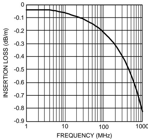
Figure 4. CAT5e Maximum Attenuation per TIA/EIA-568-B.2
