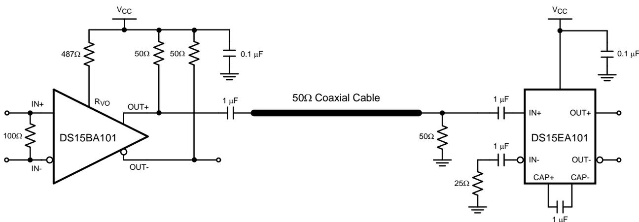
**Figure 11. Cable Extender Chipset Connection Diagram for 50Ω Coaxial Cables**
