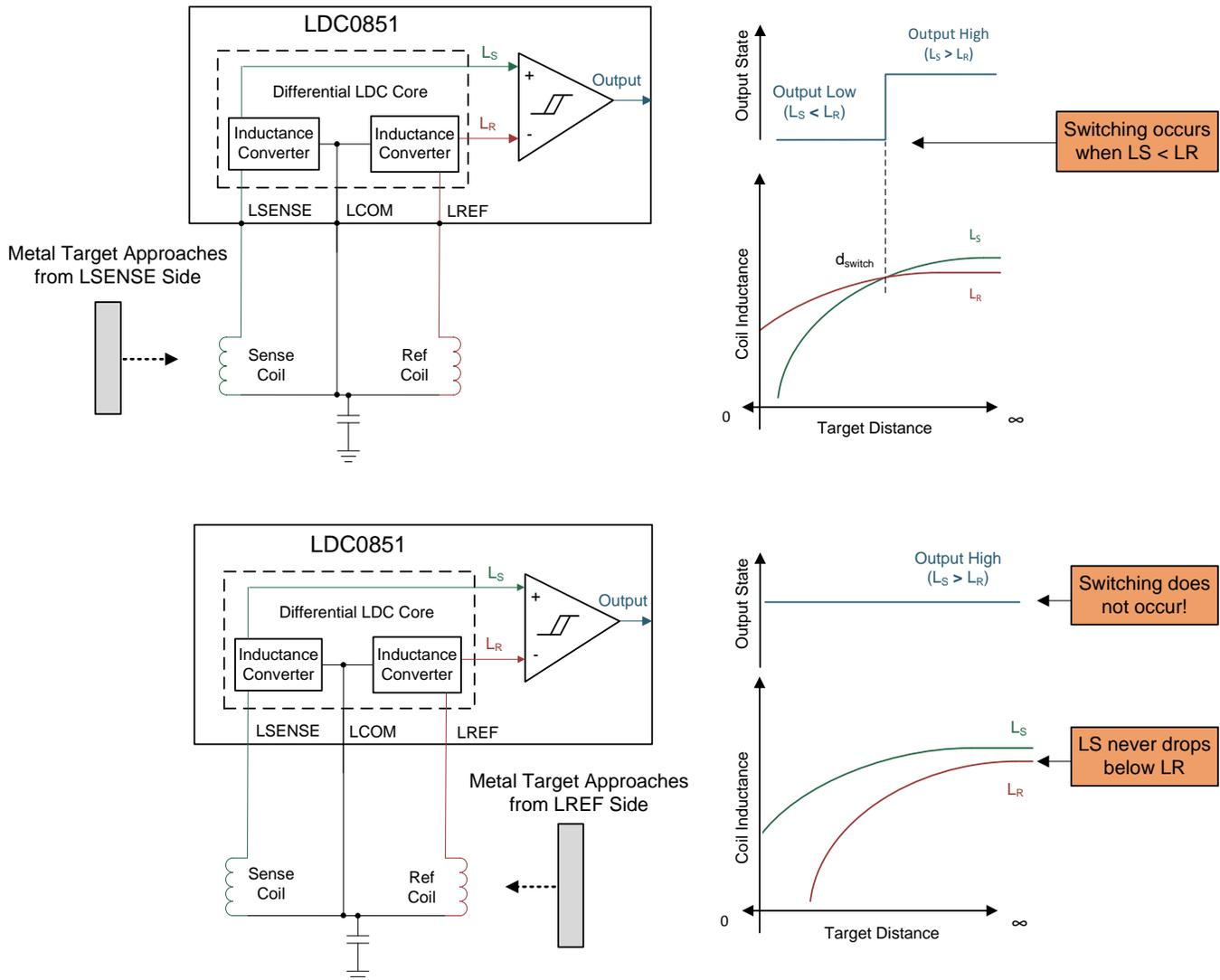
Figure 3. Unidirectional Sensing for Stacked Coils
