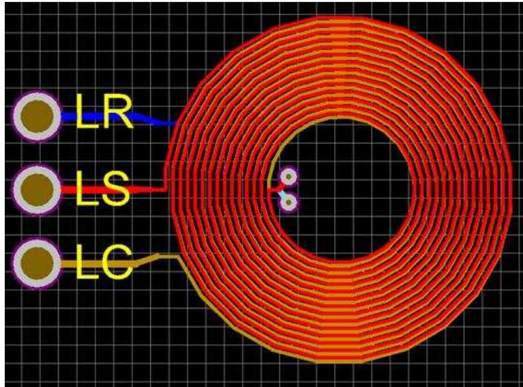
Figure 16. Example WEBENCH Coil Layout
