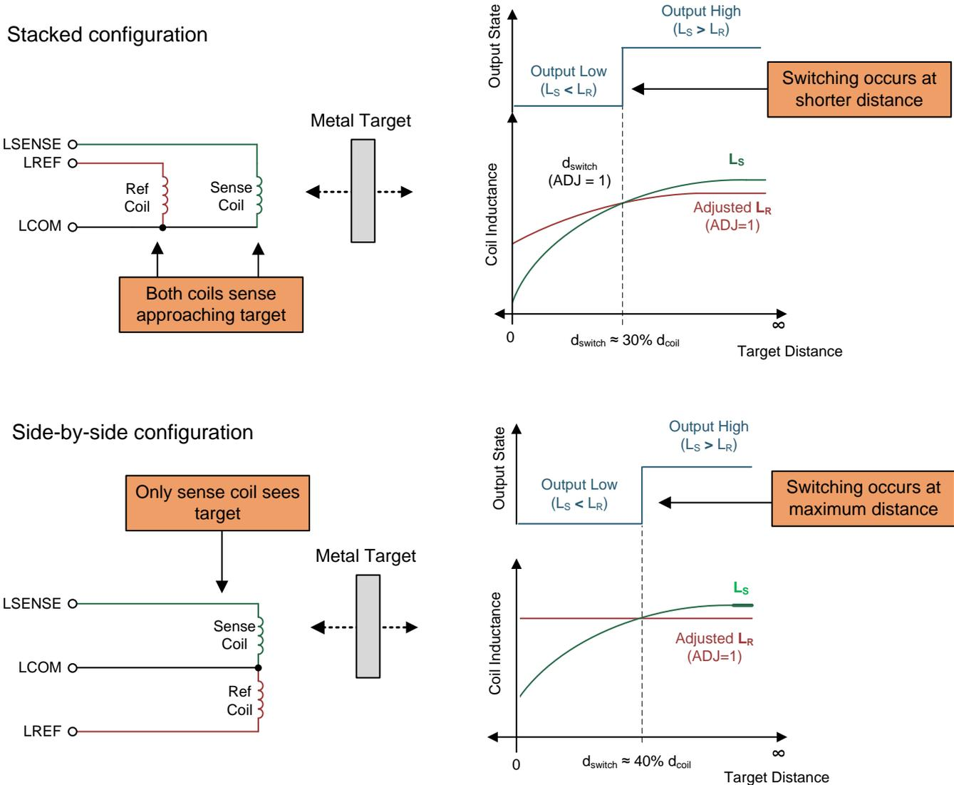
**Figure 4. Stacked vs Side-by-Side Coil Switching Distance**
