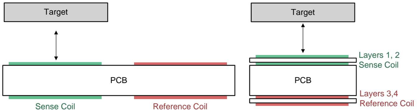
Figure 6. Number of Required PCB Layers for Side-by-Side and Stacked Coils
