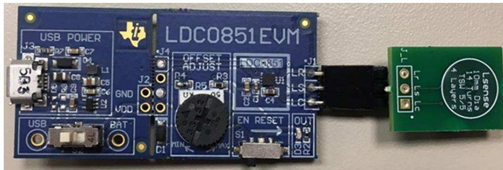
Figure 17. Prototyping Stacked Coils With LDC0851EVM
