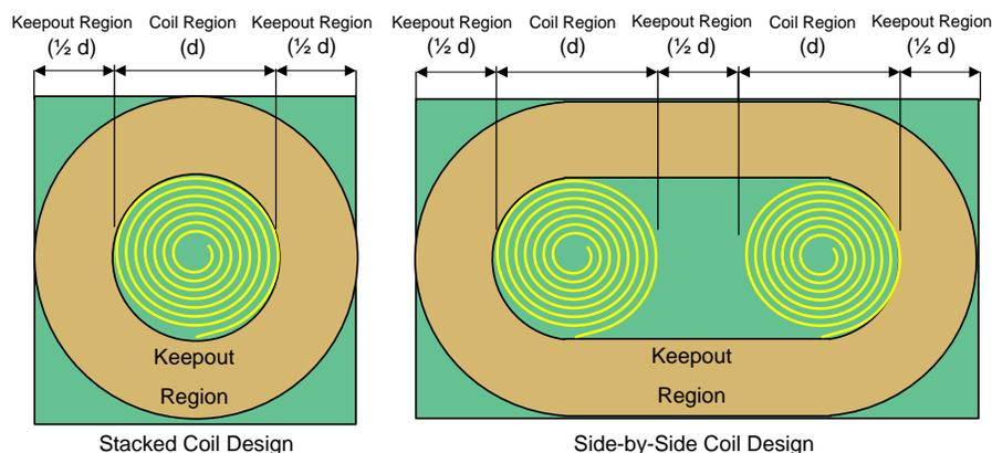
**Figure 2. PCB Area Comparison for Stacked vs Side-by-Side Coils**
