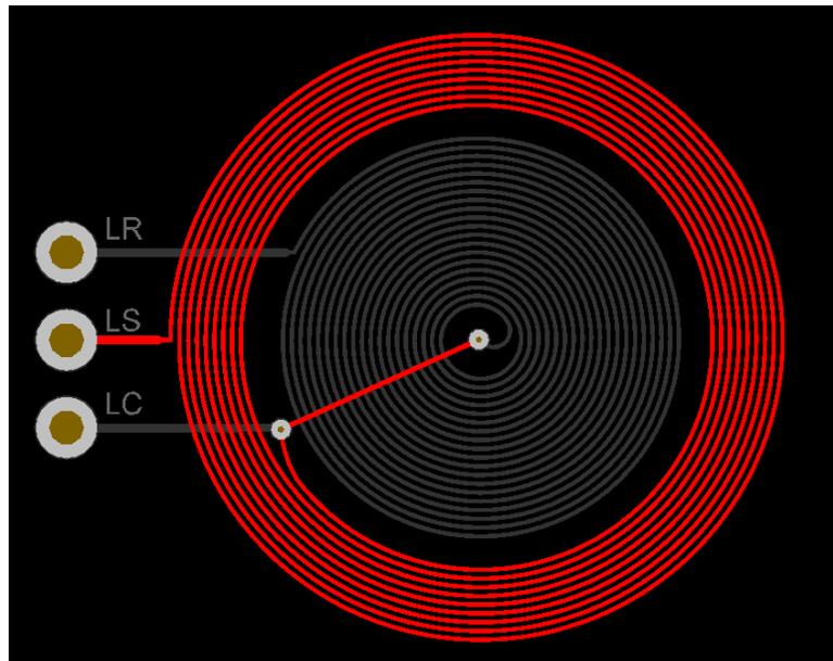
Figure 14. 2-Layer Stacked Coil, Top Layer (LSENSE)
