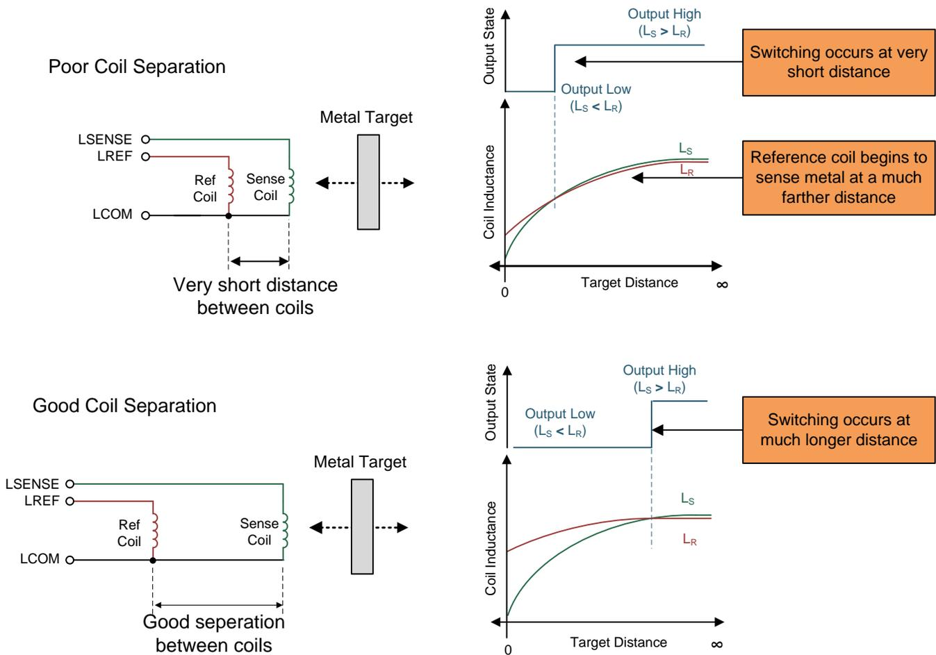
Figure 9. Effect of Poor vs Good Separation Between Coils
