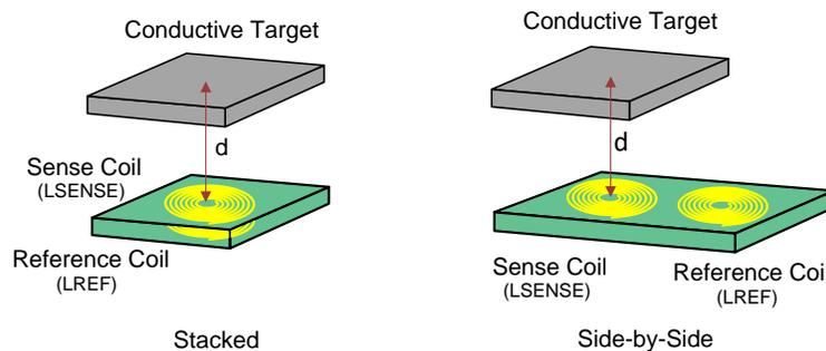
**Figure 1. Stacked and Side-by-Side Coil Arrangements**
