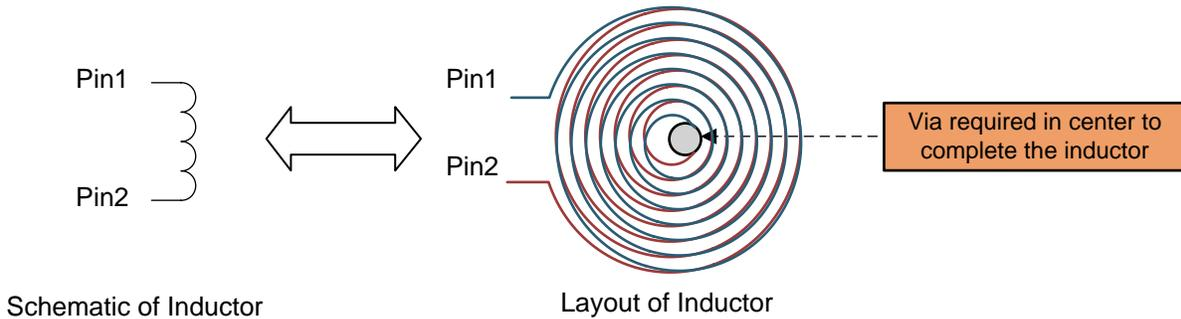
Figure 5. Schematic-Layout Equivalence of a PCB Inductor
