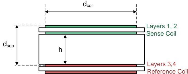
**Figure 10. Key Dimensions for Stacked Sensor PCB Construction**
