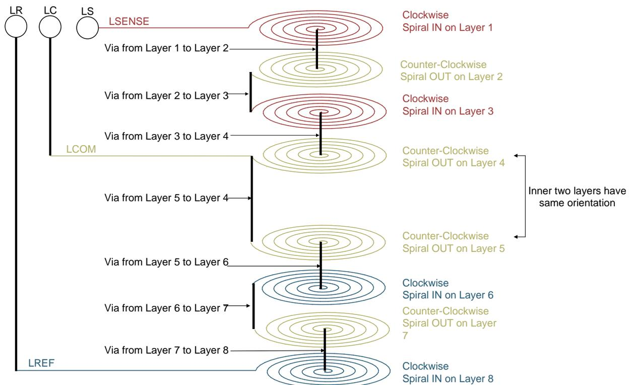
Figure 8. Stacked Coil Orientation for Eight Layers
