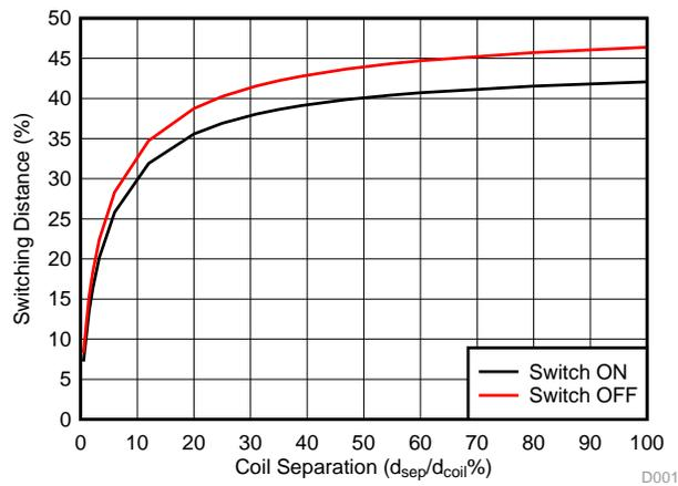
**Figure 11. Switching Distance vs. Coil Separation**
