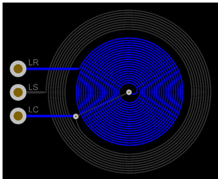
Figure 15. 2-Layer Stacked Coil, Bottom Layer (LREF)
