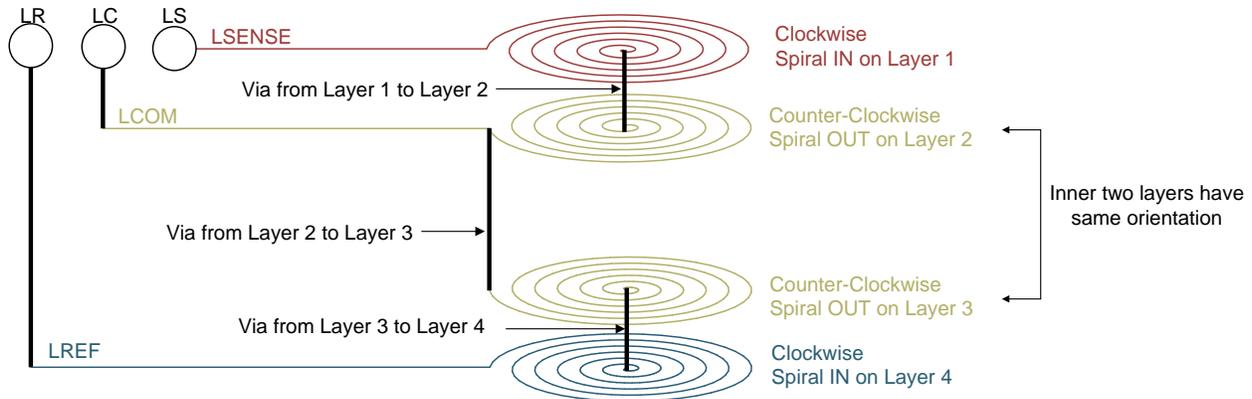
Figure 7. Stacked Coil Orientation for Four Layers
