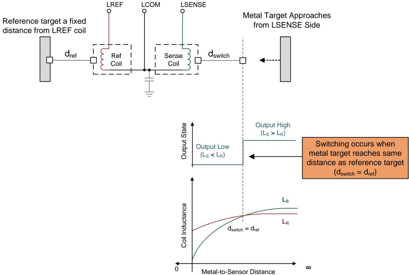
Figure 13. Fixed Distance Reference Target for Stacked Coils
