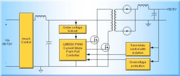
Fig. 1: Push-pull converter for VOIP applications
