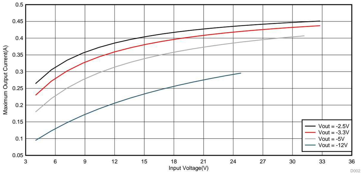
**Figure 3. Recommended Maximum Output Current for LMZM23600**
