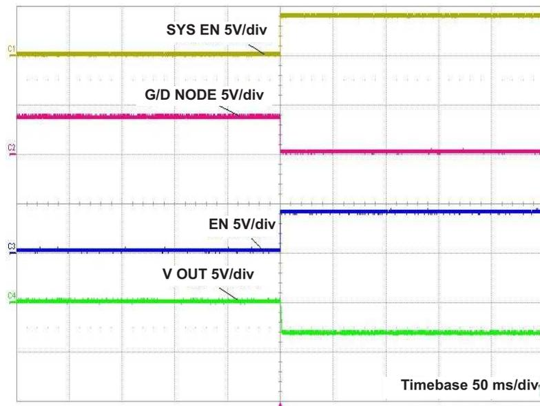
Figure 13. EN Pin Level Shifter on Start-Up
