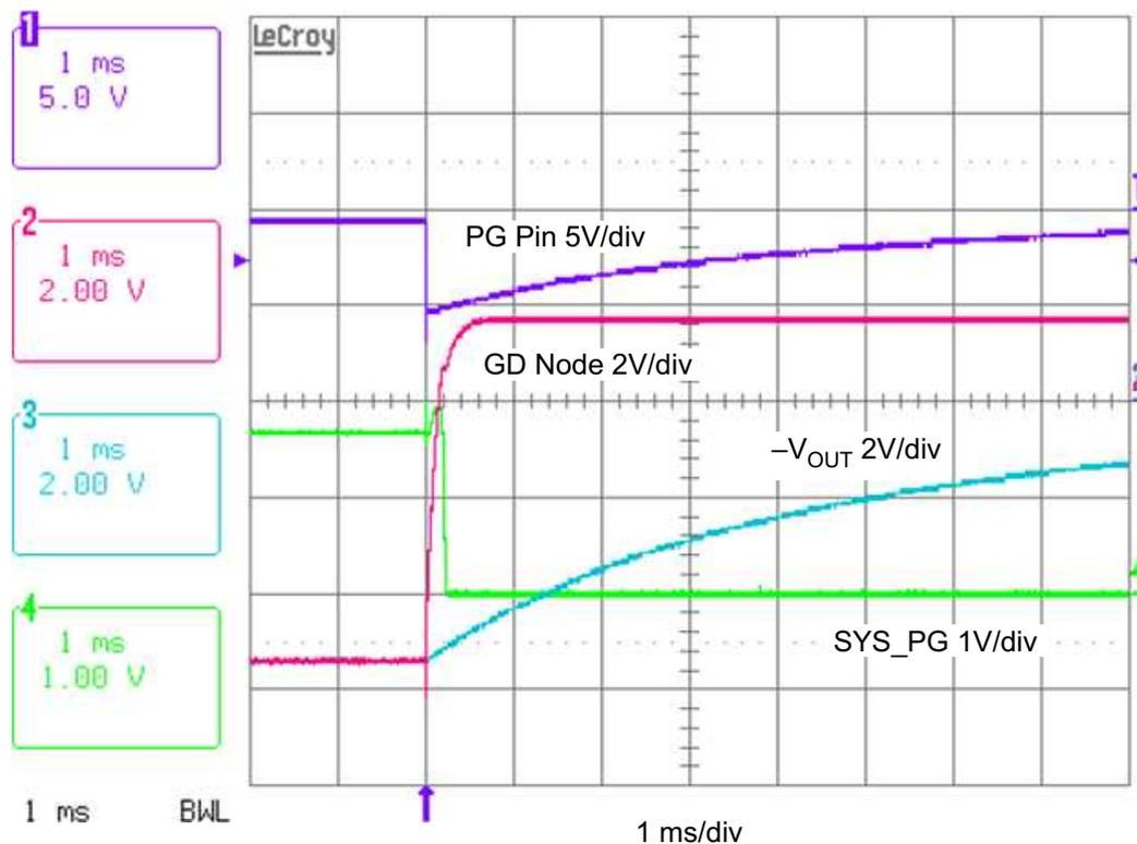
Figure 17. PG Pin Level Shifter on Shutdown
