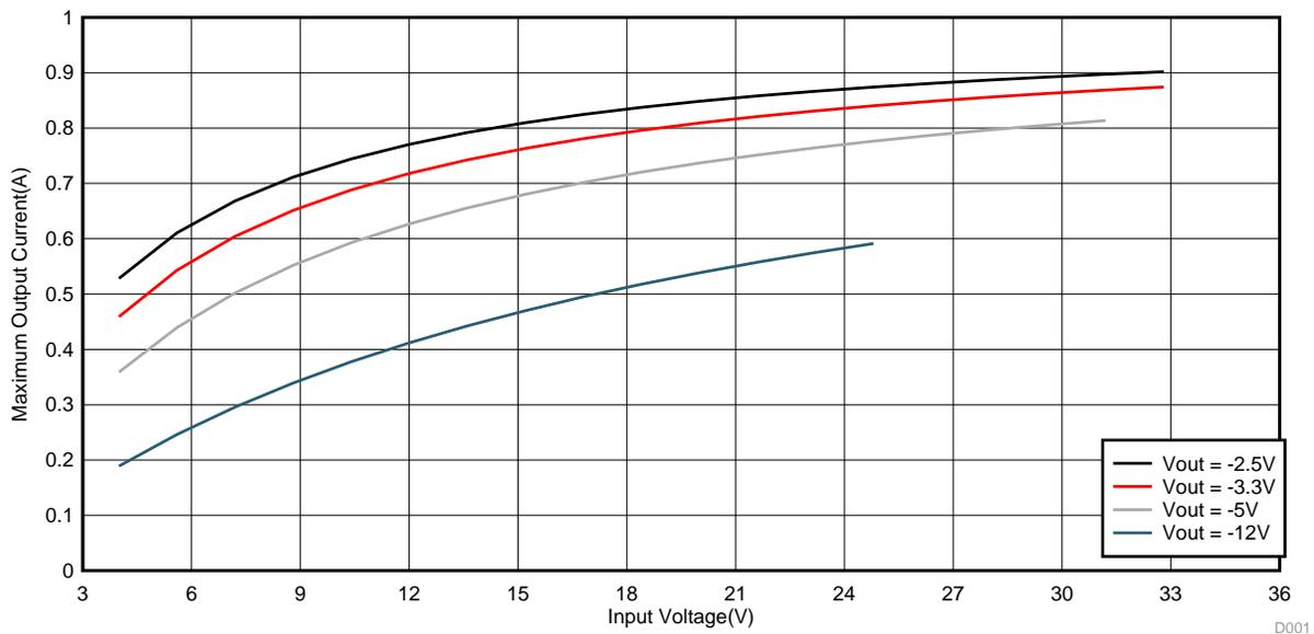
**Figure 2. Recommended Maximum Output Current for LMZM23601**
