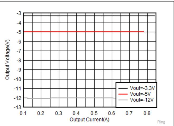
Figure 7. Load Regulation at  $V_{IN} = 24\text{ V}$
