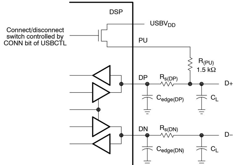
† Consult the device-specific data manual for the required values of  $R_{s(DP)}$ ,  $R_{s(DN)}$ ,  $C_{edge(DP)}$ ,  $C_{edge(DN)}$ , and  $C_L$ .
