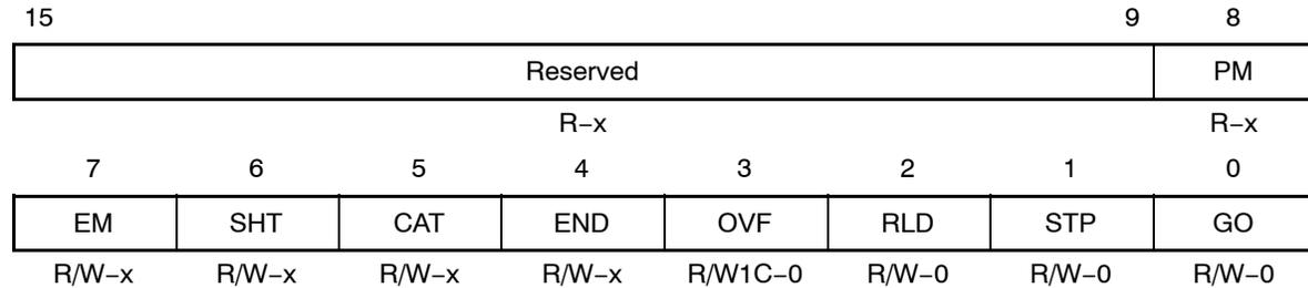
**Legend:** R = Read; W = Write; W1C = Write 1 to clear (writing 0 has no effect); -n = Value after reset; -x = Value after reset is not defined
