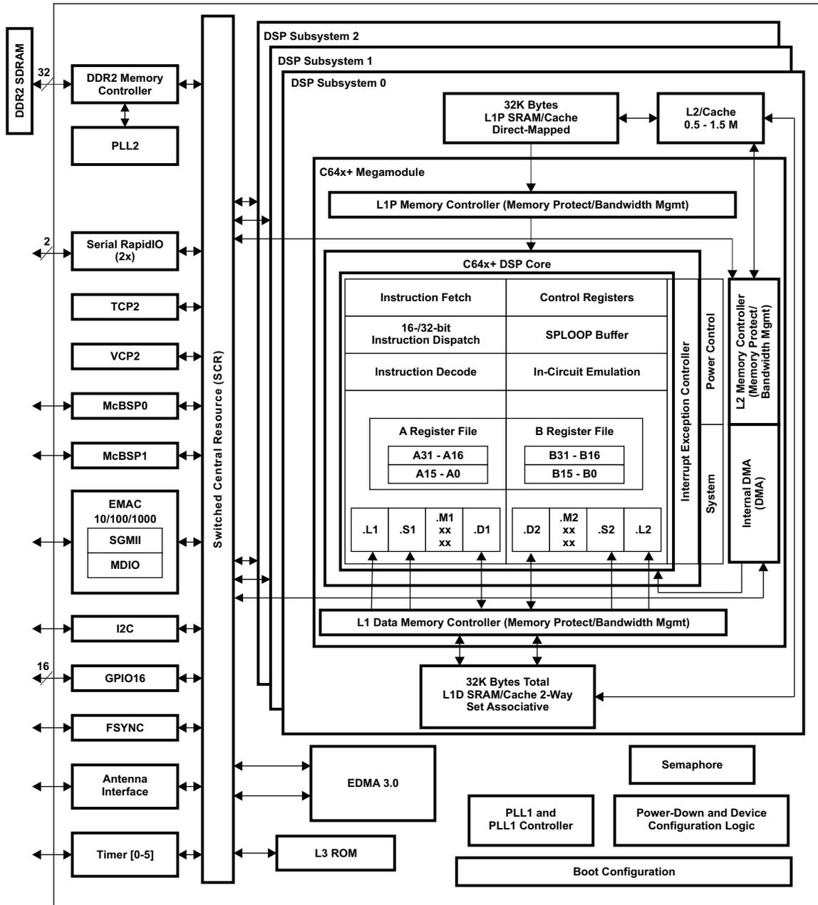
Some GPIO pins are muxed with other device pins. For details on specific muxing and for the availability of the register bits, see the *TMS320C6474 Multicore Digital Signal Processor* data manual ([SPRS552](#)). GPINT[0:15] are all available as synchronization events to the EDMA and as interrupt sources to the CPU.
