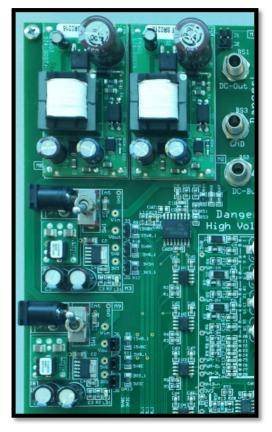
Figure 3-11. Power Supply Block
