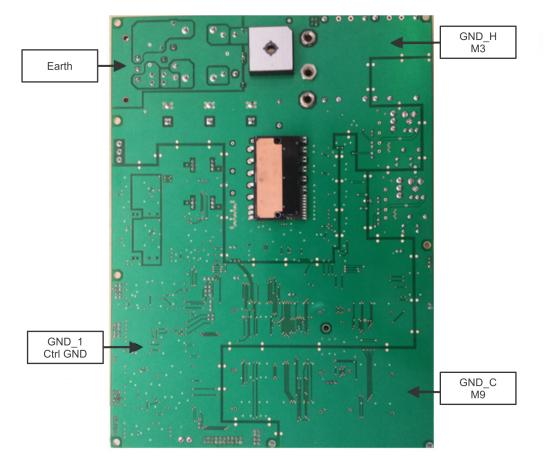
Figure 3-13. Various GND Planes on the Bottom of Board
