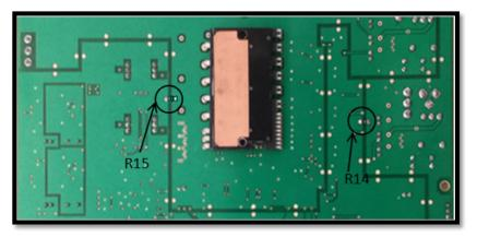
Figure 3-14. Default Connection of Various GND Planes
