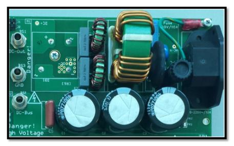
Figure 3-15. AC Line Input Filter and Rectifier
