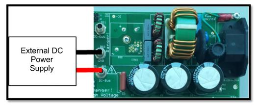
Figure 3-16. Powering Through an External DC Source
