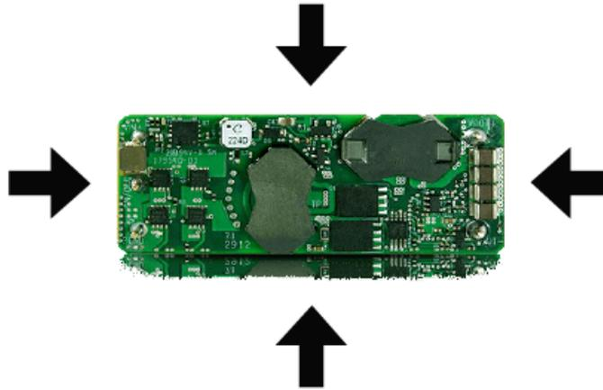
**Figure 3. DC/DC Converters with Reducing Form-factor Trends**
