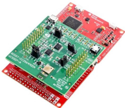
A key advantage of the CC2564MODA module is not only its ability to seamlessly interface with the MSP432 MCU, but it also delivers a turnkey solution out of the box. The module comes fully loaded with royalty-free software stacks that are compatible with the MSP432 MCU, allowing an engineer to easily add Bluetooth connectivity to a device without RF expertise.
