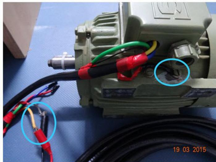
**Figure 7: A close-up of the test setup in Figure 6 (blue circles show the connection – the measurement is between the Y-terminal of the motor and earth)**
