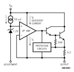
Figure 1. LM317-N Functional Schematic
