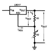
Figure 2. Typical Application Using the LM317-N
