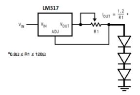
Figure 3. Constant-current LED Driver Using the LM317-N
