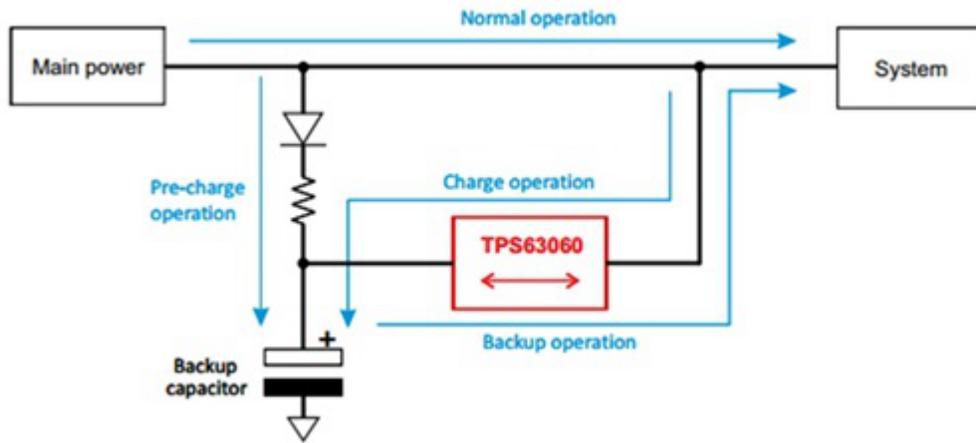
Figure 1. The **TPS63060** Provides Bi-directional Operation for Systems Which Require a Backup Power Function
