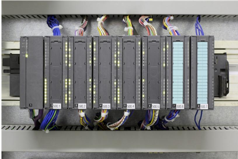
Programmable logic controllers (PLCs) are more and more common in industrial automation systems. Controlling all sorts of machines in every conceivable manufacturing environment requires programmability for various functions, from moving the valves on a mixing tank in a chemical plant to controlling the speed on conveyer belts on a manufacturing line. The same PLC card can be used for multiple, different processes; the only difference is the programmed instructions on a given PLC unit.
