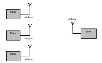
Figure 1. Wireless MBUS Communication System
