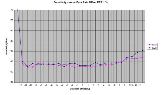
Figure 9. Sensitivity at PER 1% versus Data Rate Offset
