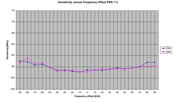
Figure 11. Sensitivity at PER 1% versus Frequency Offset
