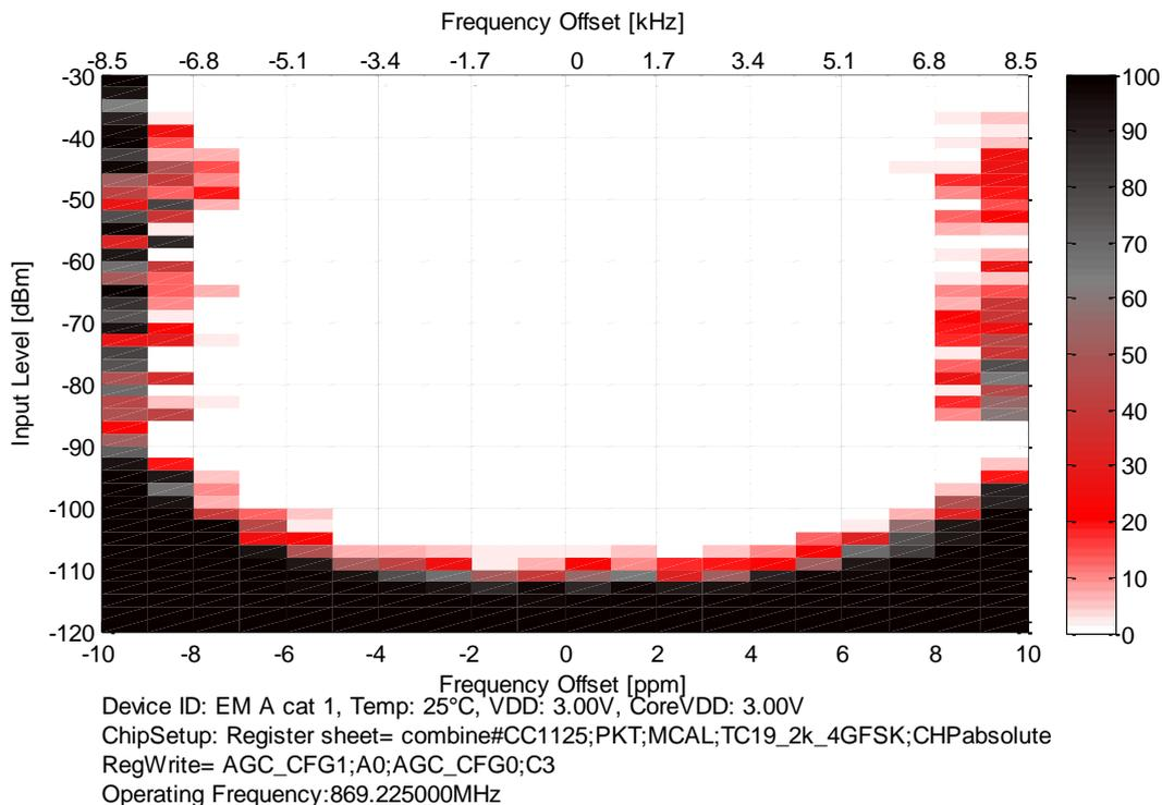
Figure 15. "Bathtub Plot". 19.2 kbit/s, 4GFSK, 25 kHz Filter Bandwidth
