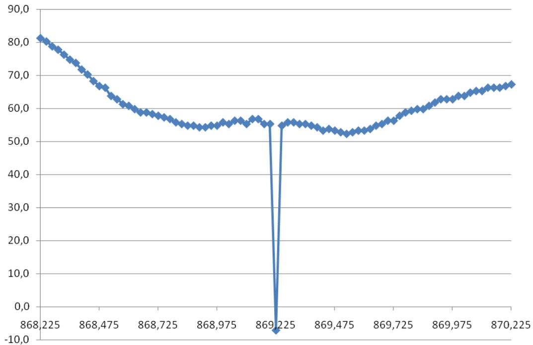
Figure 12. Spurious Response Rejection @4.8kbit/s, 16.6 kHz Filter Bandwidth with FB2PLL
