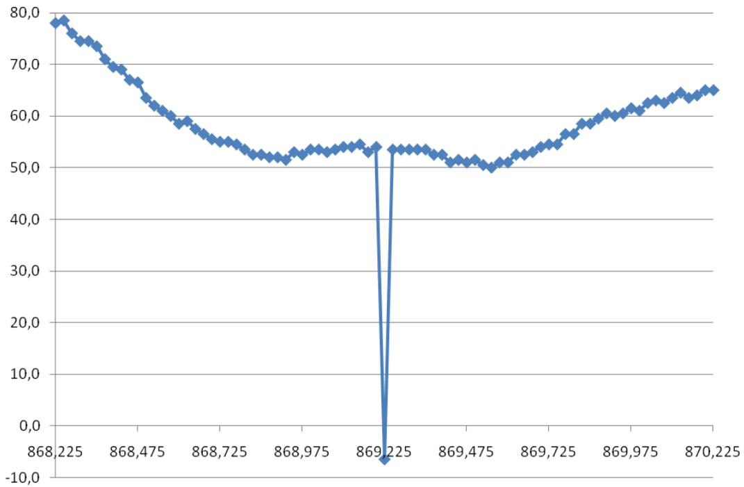
**Figure 16. Spurious Response Rejection @19.2kbit/s, 25 kHz Filter Bandwidth**
