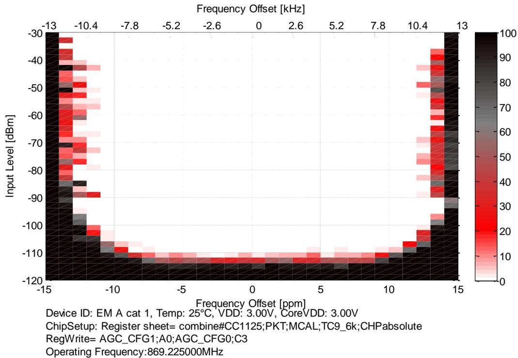
**Figure 13. “Bathtub Plot”. 9.6 kbit/s, ±4.8 kHz, 19.2 kHz Filter Bandwidth with FB2PLL**
