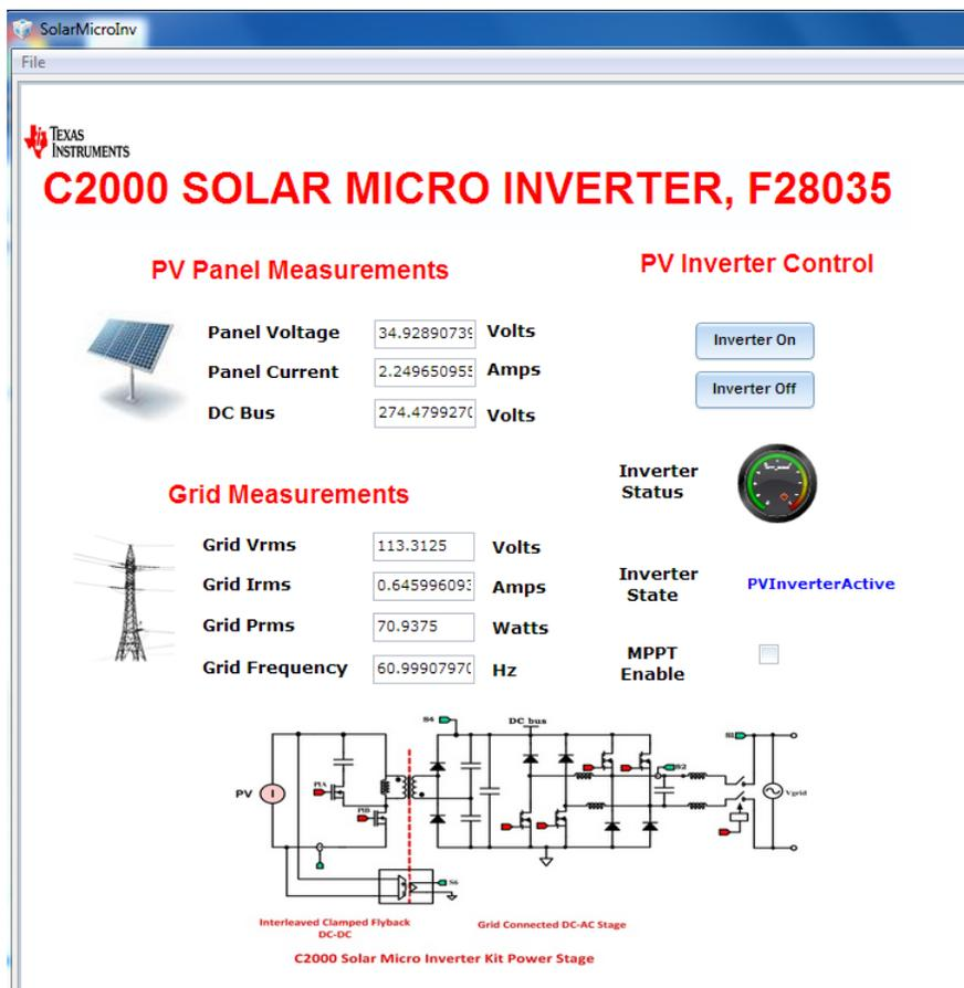
Figure 5. Solar Micro Inverter Release GUI
