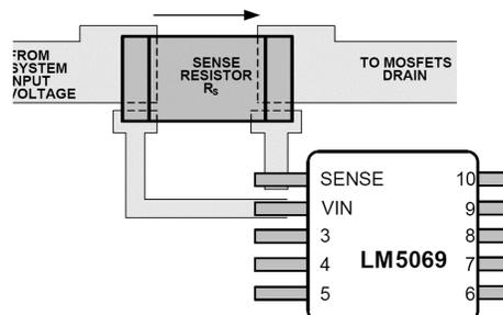
Figure 17. U1 SENSE and  $V_{IN}$  Pin Pad Connection using Resistors of Kelvin Type
