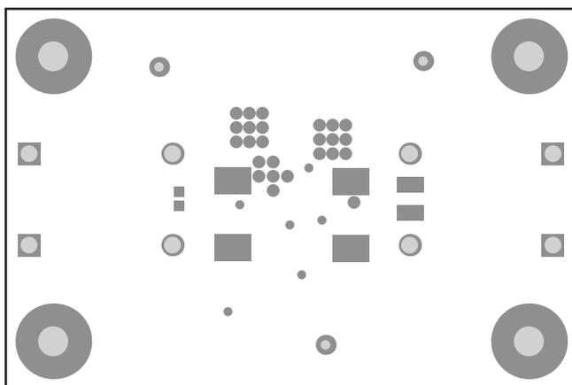
Figure 23. Bottom Solder Mask
