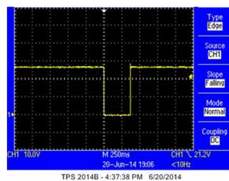
Figure 12. Output Voltage of the Protection Device during Surge at 100-Ω Load
