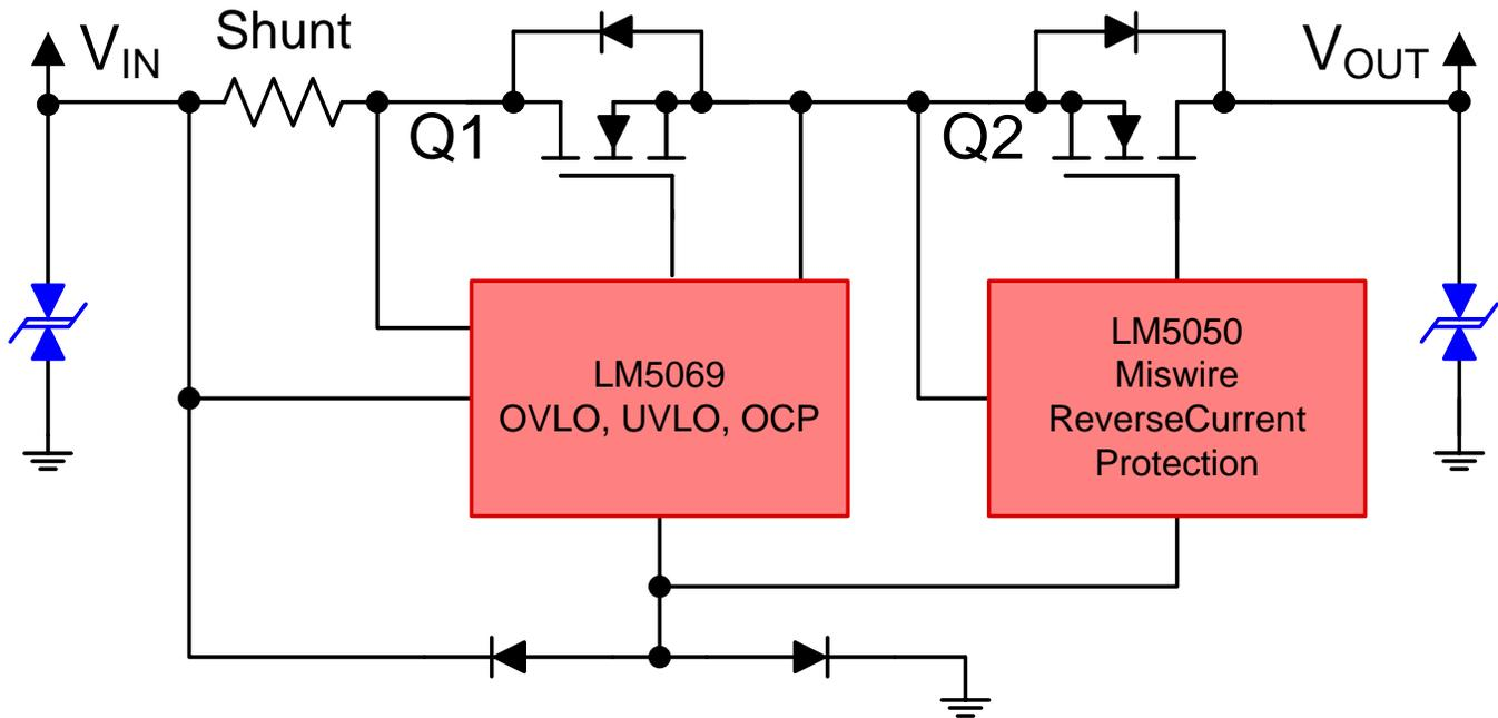
Figure 2. Simplified Block Diagram with the High Power Path between  $V_{IN}$  and  $V_{OUT}$
