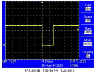
Figure 14. Output Voltage of the Protection Device during Surge at 15-Ω Load
