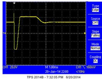
Figure 10. Output Voltage of the Protection Device during Surge at No Load
