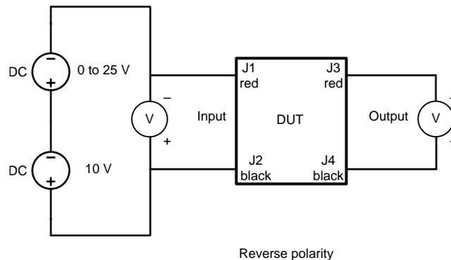
**Figure 6. Measurement Setup for Reverse Polarity Current Measurement**
