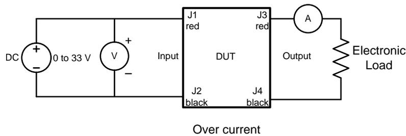
**Figure 5. Measurement Setup for Circuit Breaker Function**
