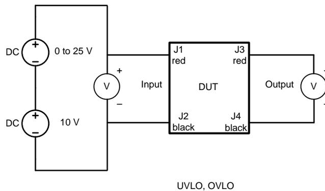
**Figure 4. Measurement setup for over and under voltage lockout**
