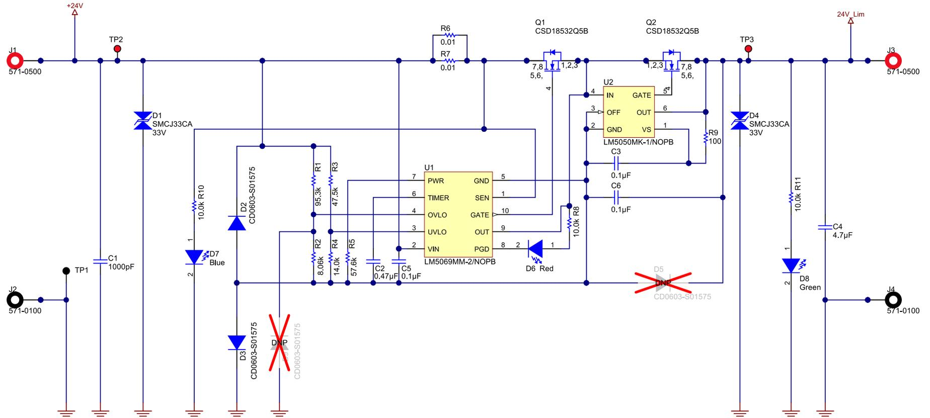
Figure 16. Schematics — Protection
