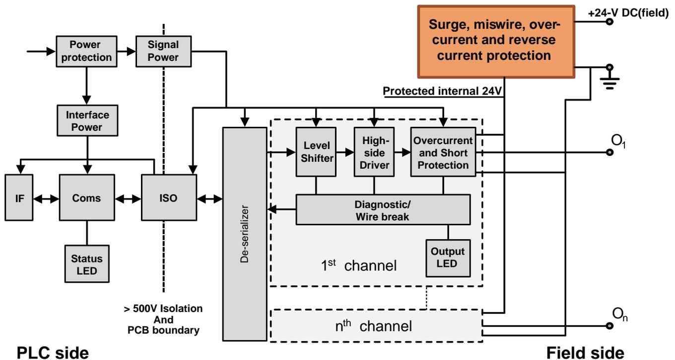
**Figure 1. Use of This Design (Orange Block) in System Context (High Side Driver with 24-V Field Supply)**
