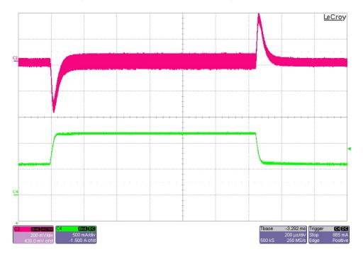
The photo below shows the output voltage (ac coupled) when the load current is stepped between 0.6A and 1.2A. Vin = 8.4V. (200mV/DIV, 500mA/DIV, 200uS/DIV)
