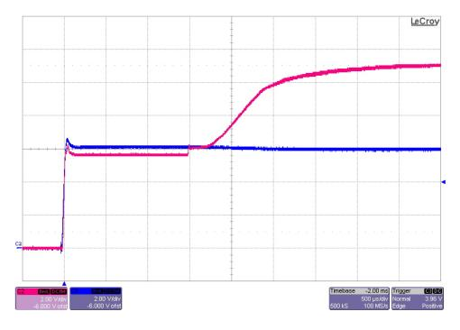
The photo below shows the output voltage startup waveform after the application of 8.4V in with the 11V output loaded to 1.2A. (2V/DIV, 500uS/DIV)
