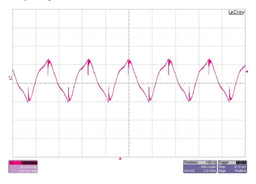
The output ripple voltage is shown in the figure below. The image was taken with the 11V output loaded to 1.2A and the input voltage set to 8.4V. (50mV/DIV, 500nS/DIV)
