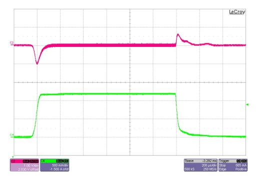
The photo below shows the output voltage (ac coupled) when the load current is stepped between 0A and 1.2A. Vin = 8.4V. (1V/DIV, 500mA/DIV, 200uS/DIV)
