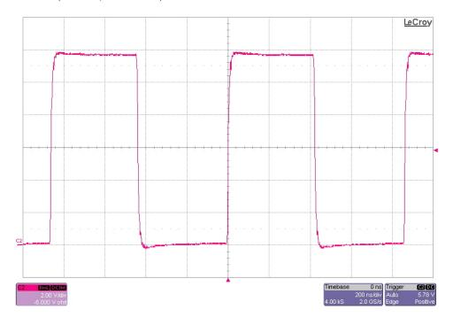
The photo below shows the switch node voltage (TP1). The input voltage is 8.4V and the 11V output is loaded to 1.2A. (2V/DIV, 200nS/DIV)
