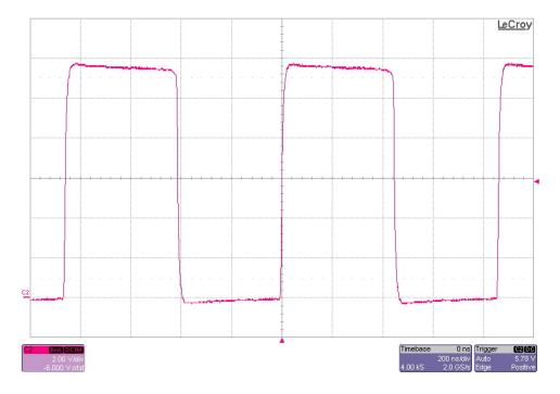
The photo below shows the switch node voltage (TP1). The input voltage is 8.4V and the 11V output is loaded to 0.180A (beginning operation in DCM). (2V/DIV, 200nS/DIV)
