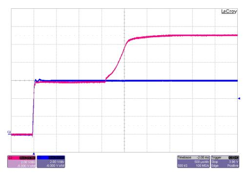
The photo below shows the output voltage startup waveform after the application of 8.4V in with the 11V output loaded to 0A. (2V/DIV, 500uS/DIV)
