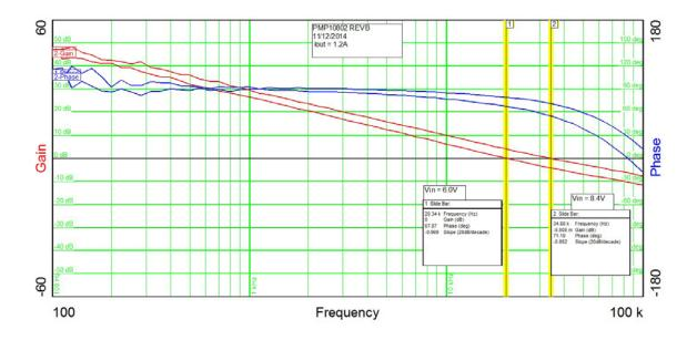
The plot below shows the boost converter's loop gain and phase margin when the 11V output is loaded to 0.25A.
