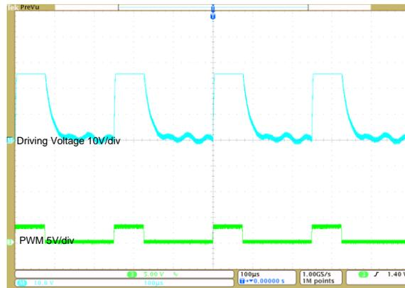
**Figure 6: Operating Waveform with 4-KHz PWM**
