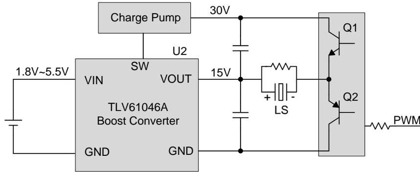
**Figure 2: Block Diagram of ±15-V Driver Circuit**
