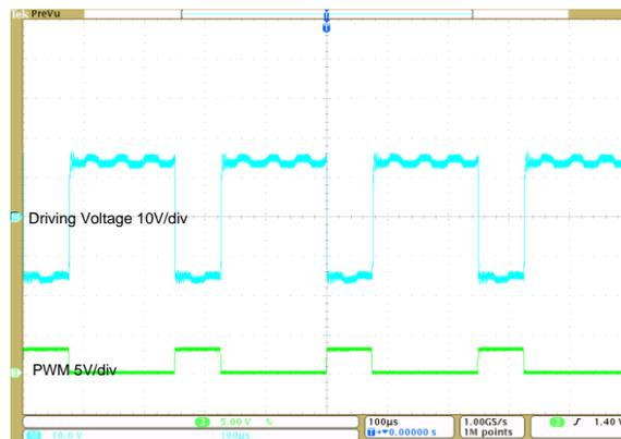
**Figure 8: Operating Waveform with 4-KHz PWM**
