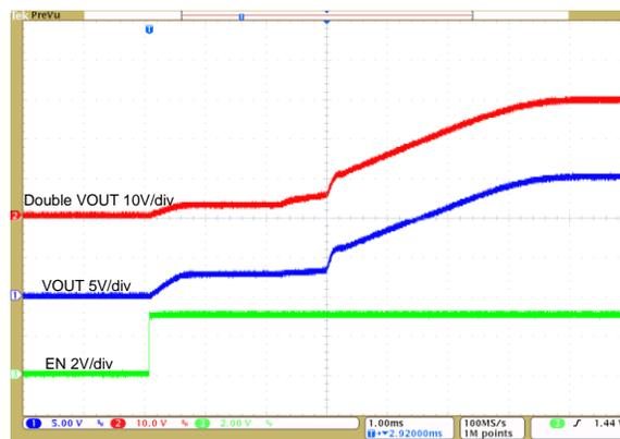
**Figure 7: Startup at VIN=3.3V**
