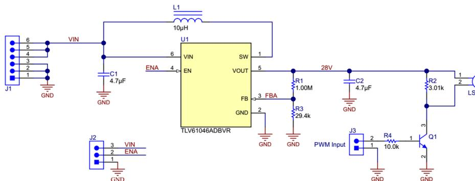
**Figure 3: 28-V Rectangular Waveform Driver Circuit**
