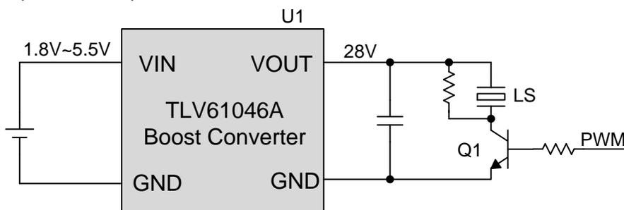
**Figure 1: Block Diagram of the 28-V Driver Circuit**
