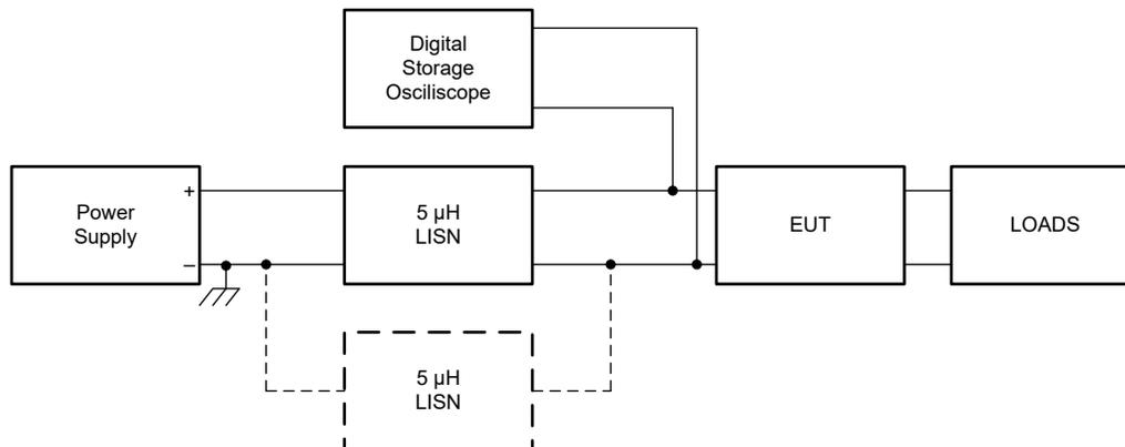
Figure 3-2. Emitted Spike Test Setup
