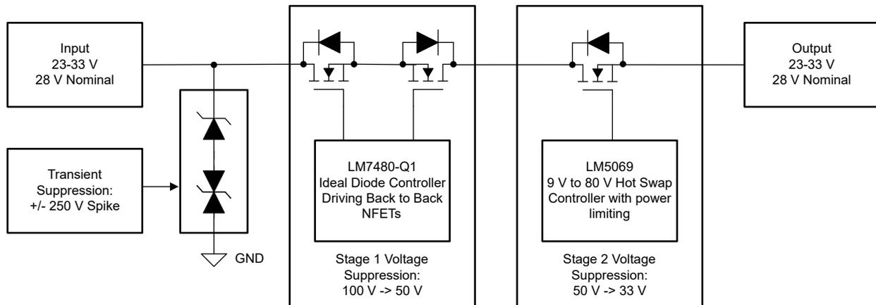
Figure 2-1. MIL-STD-1275E Protection Block Diagram
