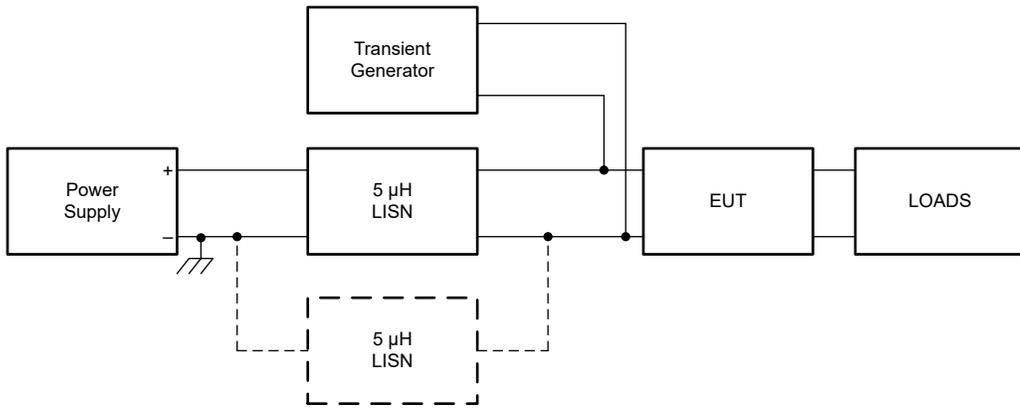
**Figure 3-3. Injected Spike Test Setup**
