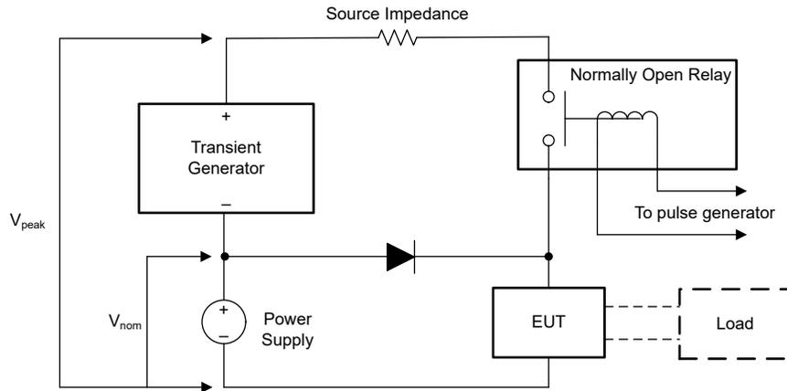
**Figure 3-4. Surge Test Setup**
