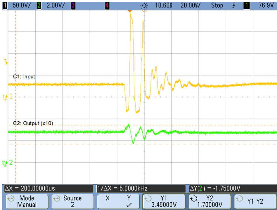
Figure 3-7. +250-V Injected Voltage Spike
