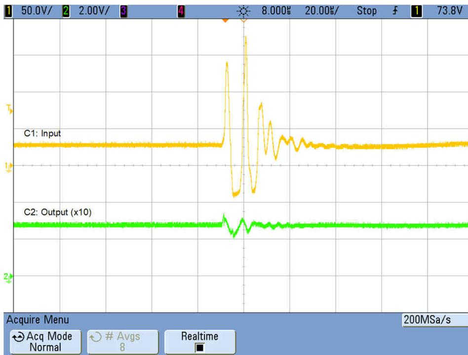
Figure 3-8. -250-V Injected Voltage Spike Event
