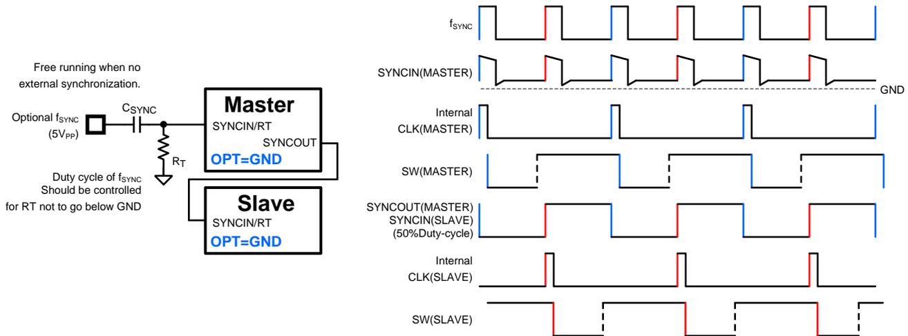
Figure 32. Dual Phase Configuration and Timing Diagram
