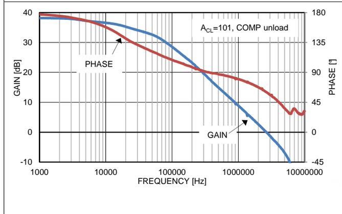
Figure 9. Error Amplifier Gain and Phase vs Frequency
