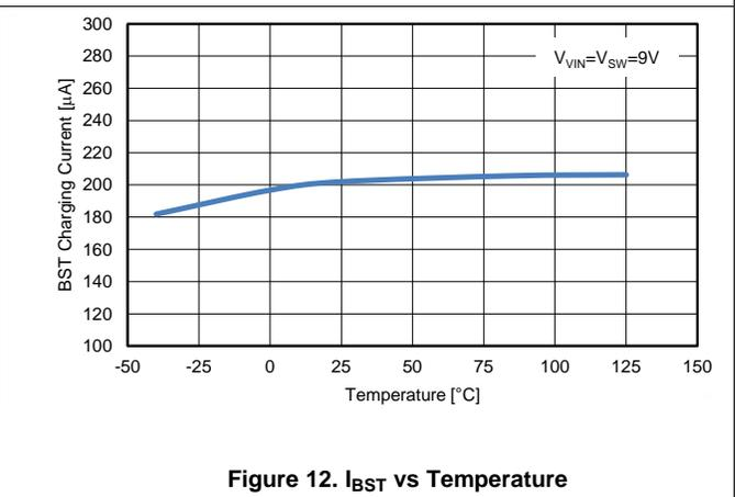
Figure 12.  $I_{BST}$  vs Temperature
