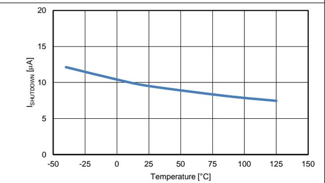
Figure 6.  $I_{SHUTDOWN}$  vs Temperature
