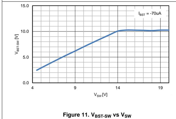
Figure 11.  $V_{BST-sw}$  vs  $V_{SW}$
