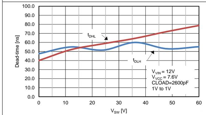
Figure 5. Dead Time vs  $V_{SW}$
