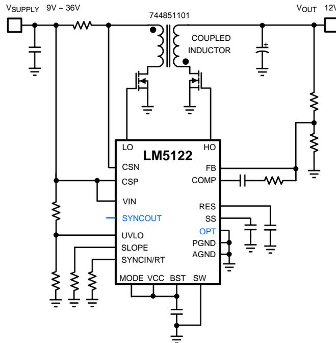
Figure 38. Non-Isolated Synchronous Flyback Converter Simplified Schematic
