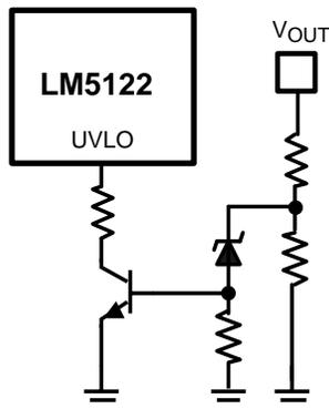
Figure 36. Output Overvoltage Protection
