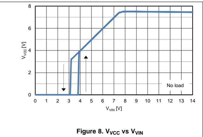
Figure 8.  $V_{VCC}$  vs  $V_{VIN}$
