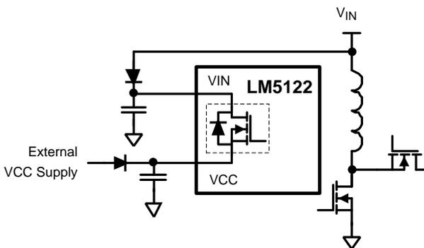
Figure 19. VIN Configuration when  $V_{VIN} < V_{VCC}$
