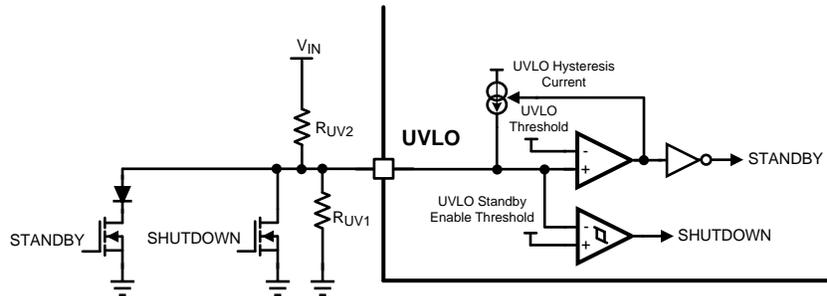
Figure 16. UVLO Remote Standby and Shutdown Control
