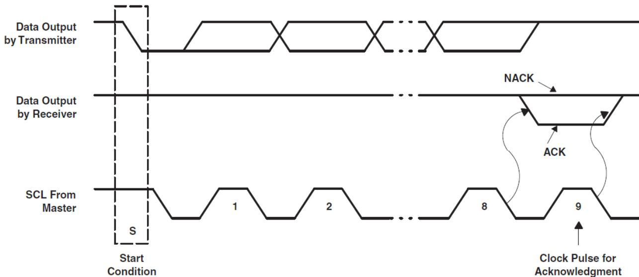
图 18. Acknowledge and Not Acknowledge on I<sup>2</sup>C Bus
