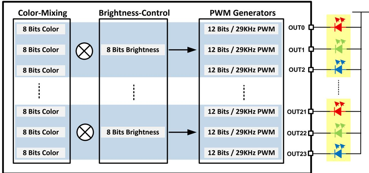
图 9. PWM Control Scheme for Each Channel
